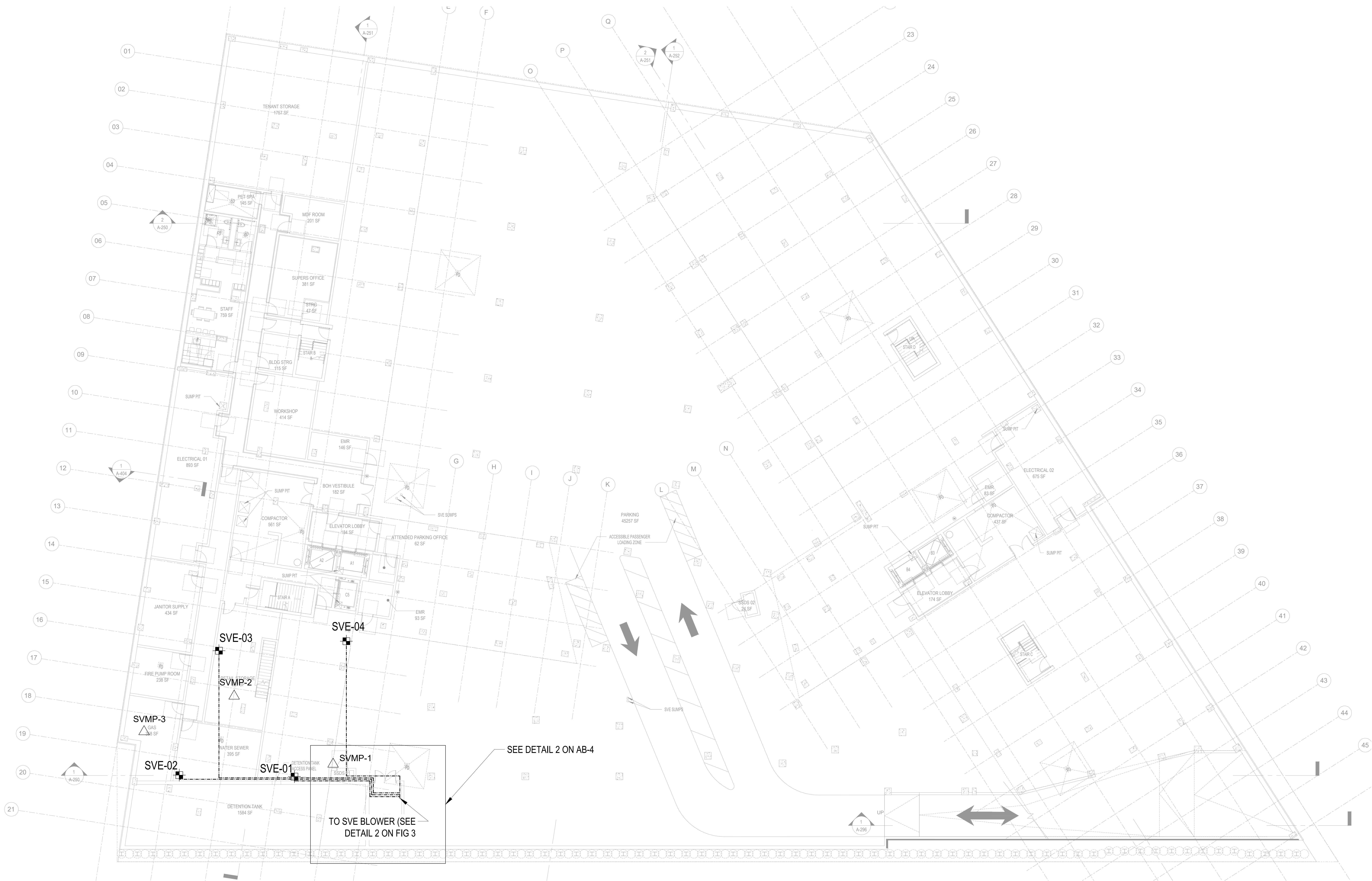
1 FIG 3 SOIL VAPOR EXTRACTION SYSTEM AS- BUILT LAYOUT
