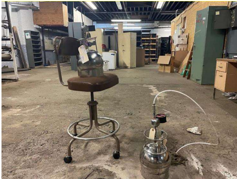
Photo 2: View of co-located sub-slab vapor and indoor air sample collection at sub-slab vapor point SSV19 (facing southwest).
