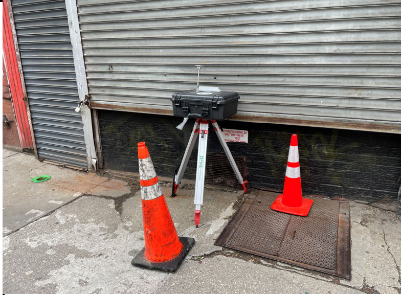
Photo 1: View of the downwind CAMP station setup.
