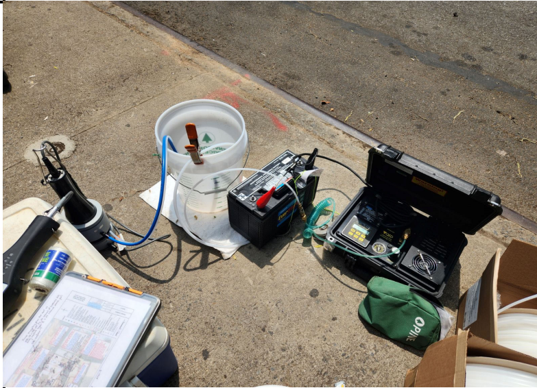
Photo 2: View of the purging setup at MW-7.
