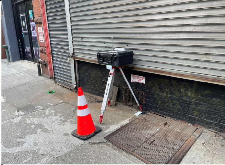
Photo 1: View of the downwind CAMP station setup.
