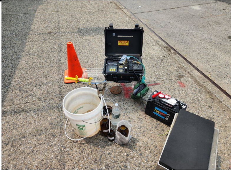
Photo 1: View of the groundwater sampling setup at MW-2.
