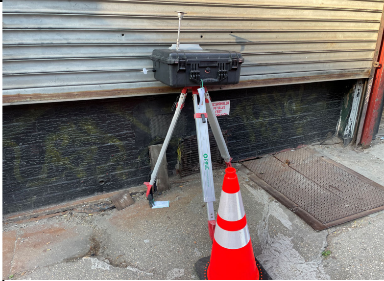
Photo 1: View of the downwind CAMP station setup.
