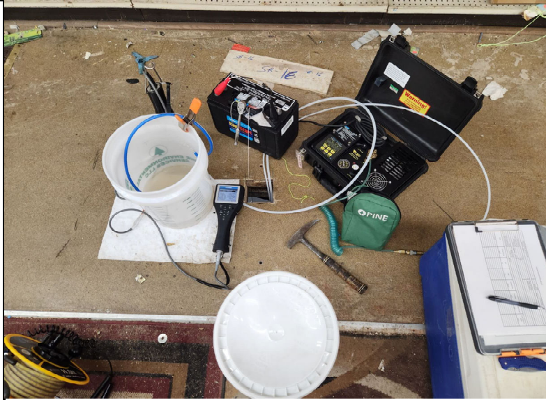
Photo 1: View of purging setup at MW-6.
