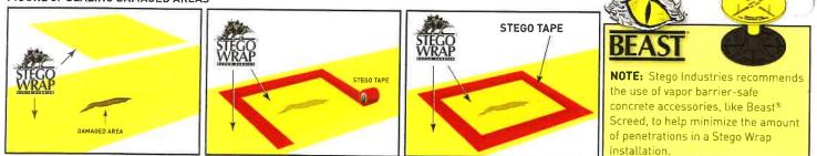
**IMPORTANT: ALL PENETRATIONS MUST BE SEALED.** All pipe, ducting, rebar, wire penetrations and block outs should be sealed using Stego Wrap, Stego Tape and/or Stego Mastic **(See Figure 4a)**. If penetrations are encased in other materials, such as expansive materials like foam, unless otherwise specified, Stego Wrap should be sealed to the underlying penetration directly.
