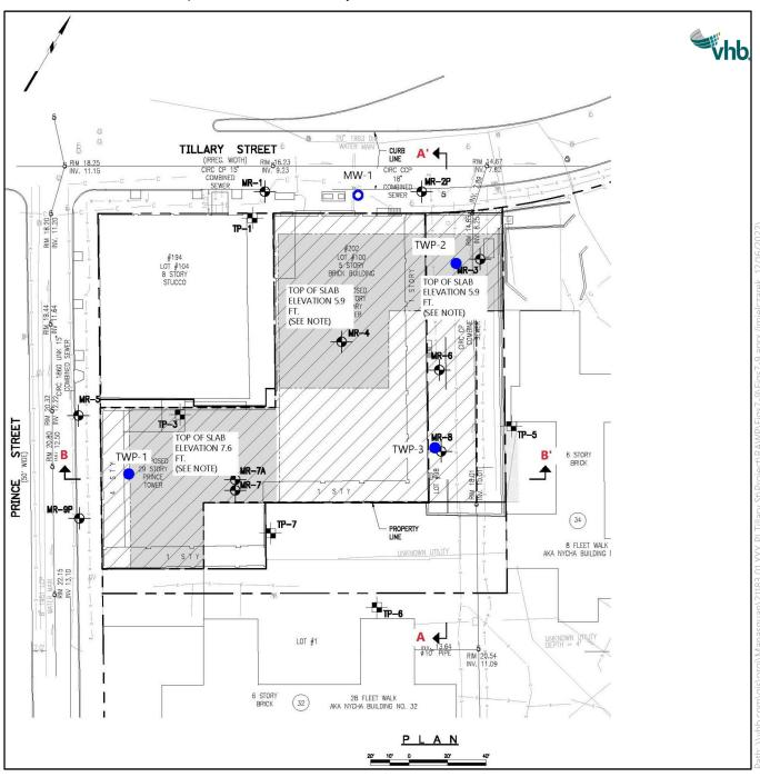
APPROXIMATE LOCATION OF PERMANENT MONITORING WELL MW-1 (INSTALLED JULY 2022)
