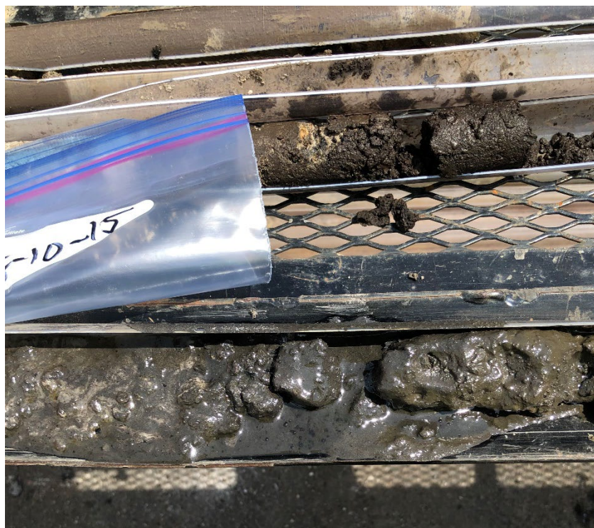
Photograph 2: Oil globules noted at GP-18 (10-15 ft. bg.).
