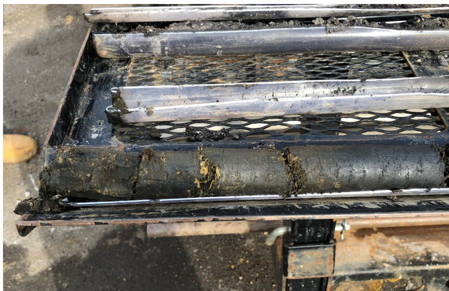
Photograph 6: Peat layer at approximately 14 feet below grade.
