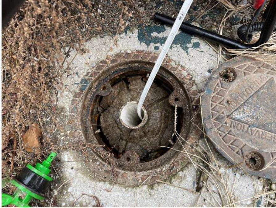
Photo 1: Langan gauging depth to groundwater from top of casing at MW01 (facing down).
