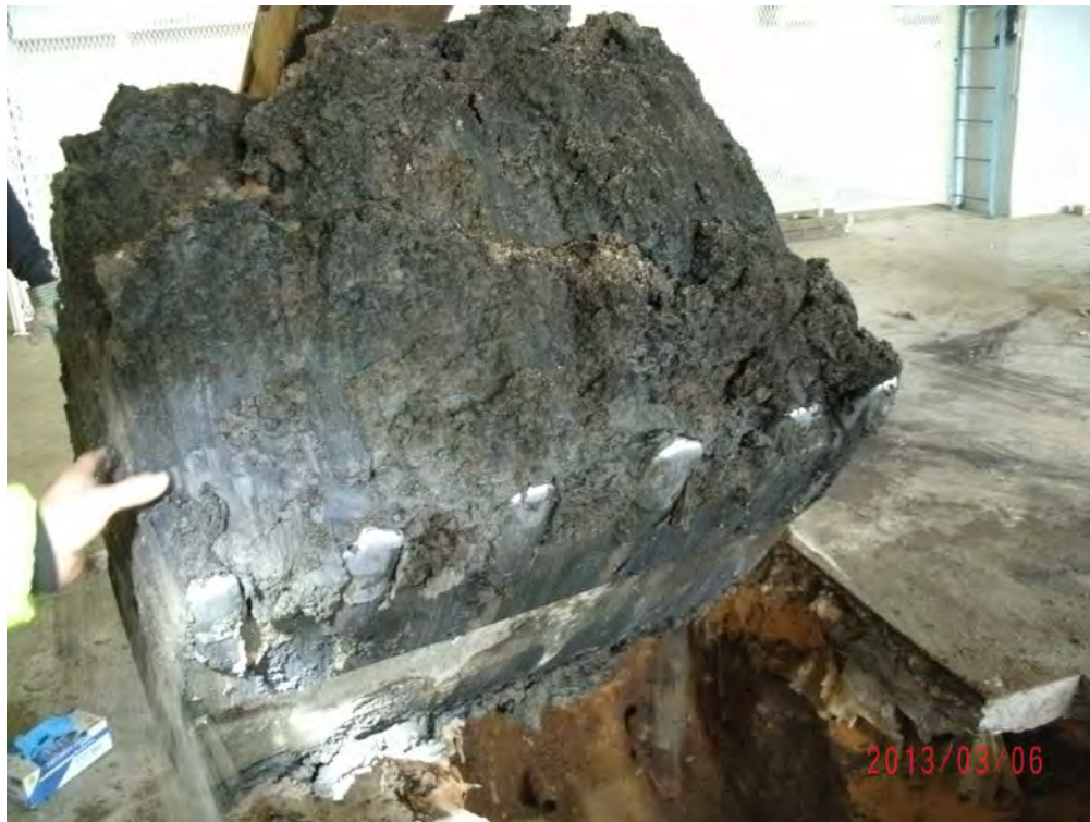
Photograph 7: Native appearing soil consisting of clay intermixed with fine sand and marsh organics at 11-feet below grade.
