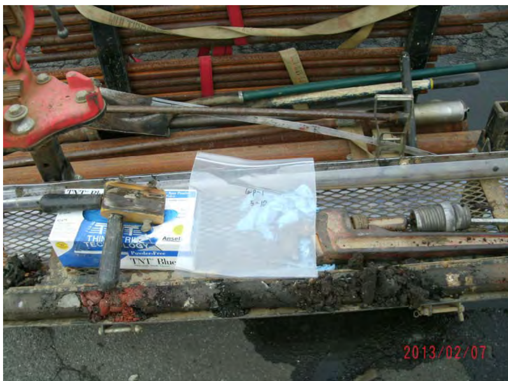
Photograph 2: Urban fill identified at GP-1 consisting of wood, brick and organics.
