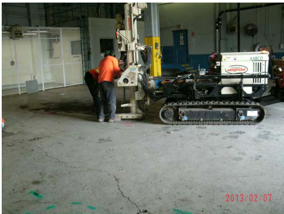
Photograph 5: Installation of GP-3 within concrete patch in garage.
