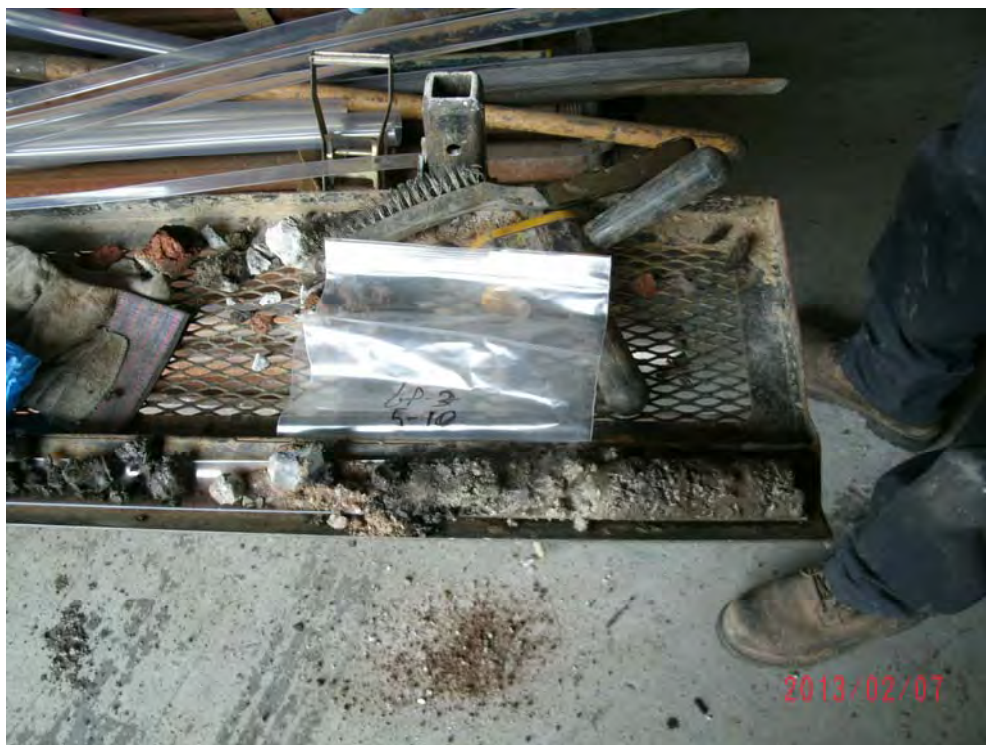
Photograph 6: Urban fill identified at GP-3.
