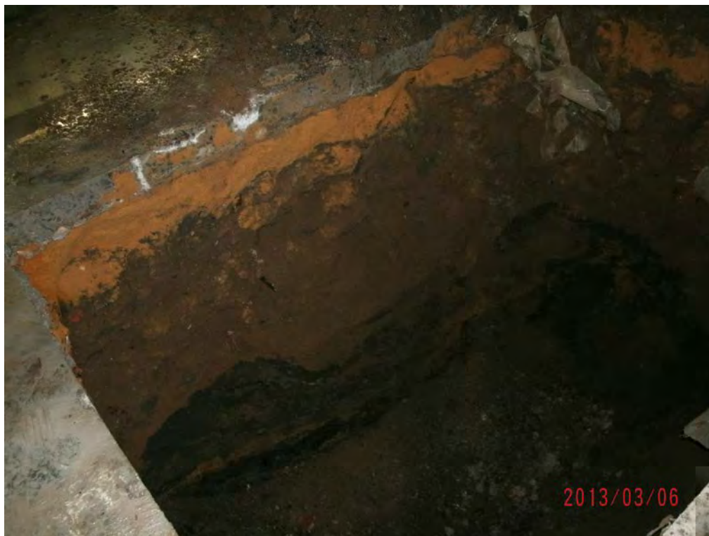
Photograph 5: Layers of urban fill observed.
