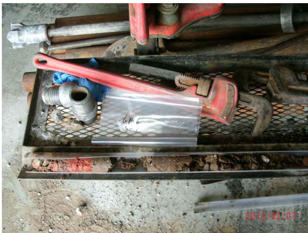
Photograph 12: Urban fill identified at GP-6.
