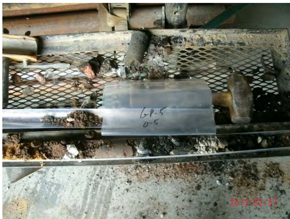
Photograph 10: Urban fill identified at GP-5.
