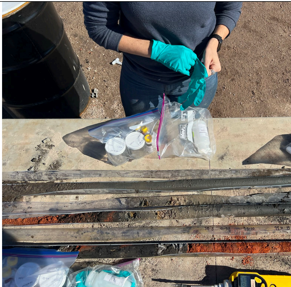
Photo 5 – Photo of material from SB-8 at the 0-5', 5-10', 10-15', and 15'-20' intervals.
