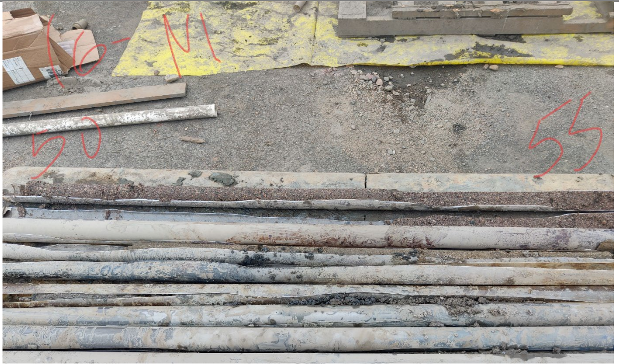
Photo 3- View of SB-16-N1 at the 50-55' interval which consisted of coarse sand.
