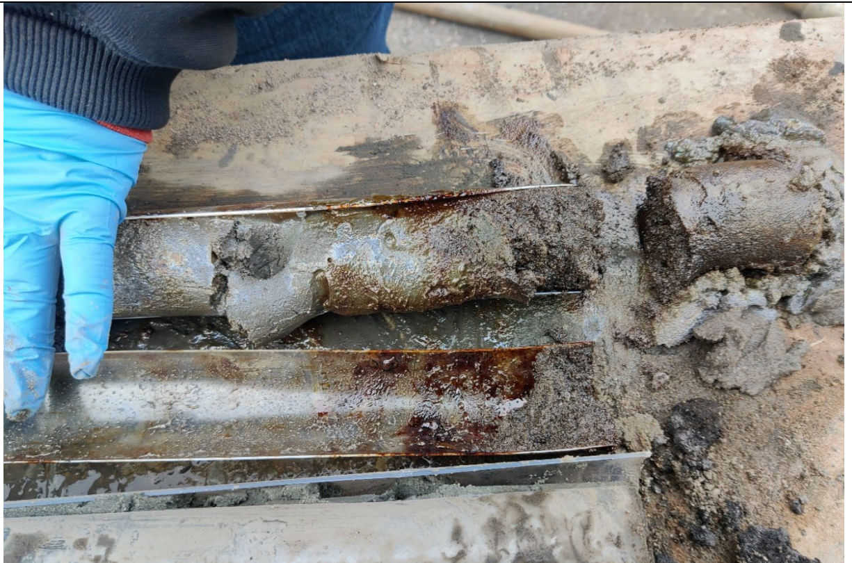
Photo 2 – View of GCM identified in SB-16-N1 at the 34-35' interval.
