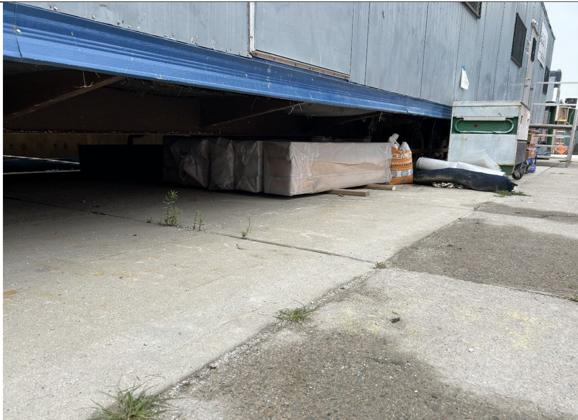
Photo 2 – Representative photo of ISS QA/QC cores stored underneath trailer and wrapped with plastic.
