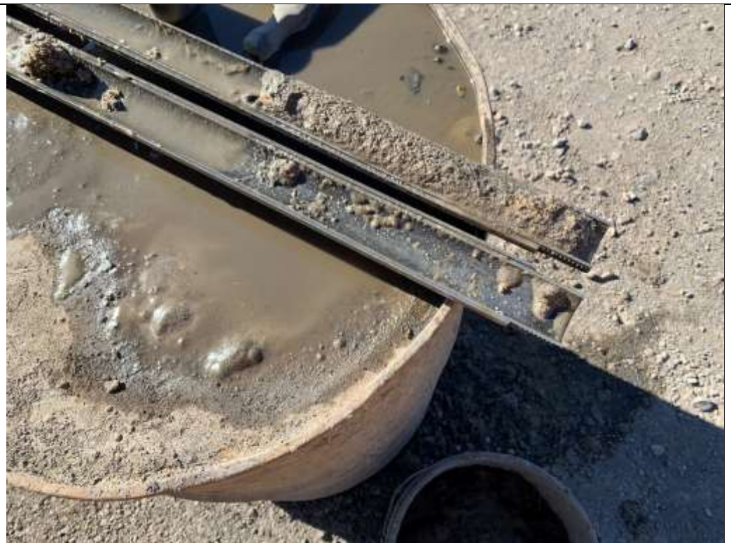
Photo 2 – Split spoon sample at B-4.
