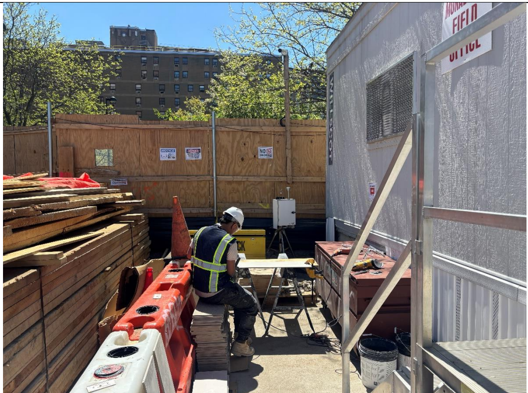
Photo 4 – Downwind CAMP station, facing south. Laborer observed grinding ceramic tile during CAMP exceedance.
