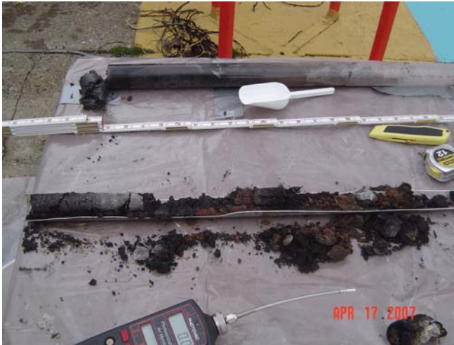
Photo #1 KSF-SB-01, (0-4') Typical fill material
