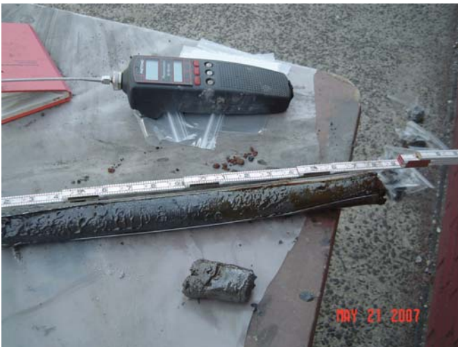
Photo#9 KSF-SB-22 (8-12') Coal tar saturated silty sand & gravel from 9' to 11.5'
