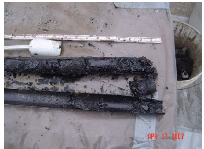
Photo#4 KSF-SB-05, (8-12') Coal tar saturated silty sand and gravel
