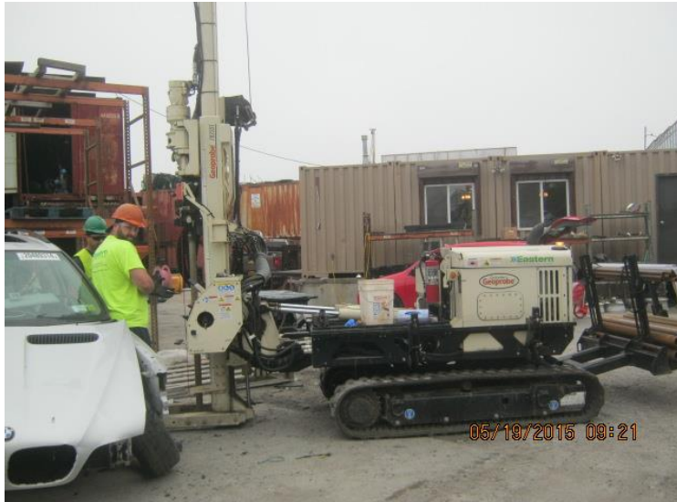
Photograph 1. Geoprobe drilling at soil boring SB-1.
