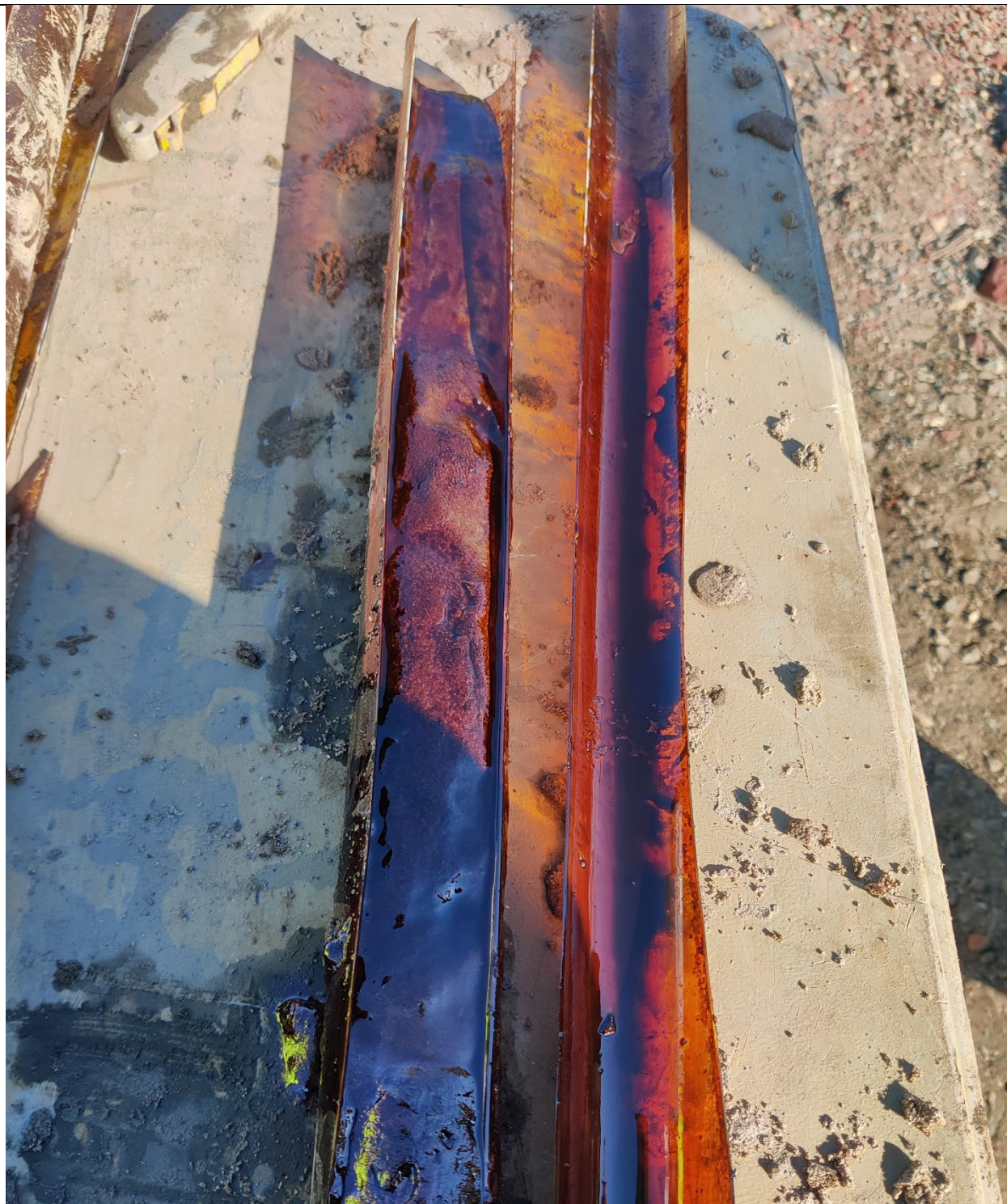
Photo 4-View of DB-1 at the 40-43; interval, saturated in MGP Coal Tar.
