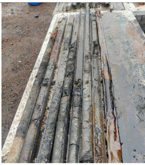
Photo 3-Additional photo of boring DB-19 at the 35-40' interval, impacted with MGP Coal Tar.
