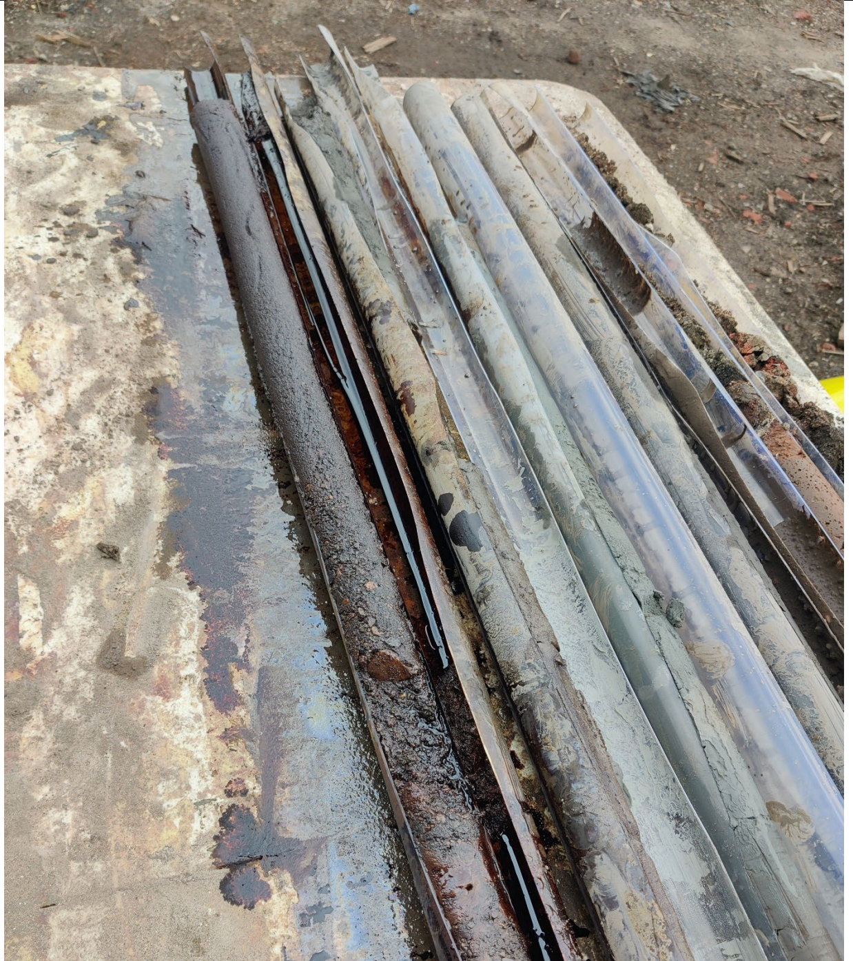
Photo 3- Additional photo of boring DB-21 impacted with MGP Coal Tar at the 35-40' interval.
