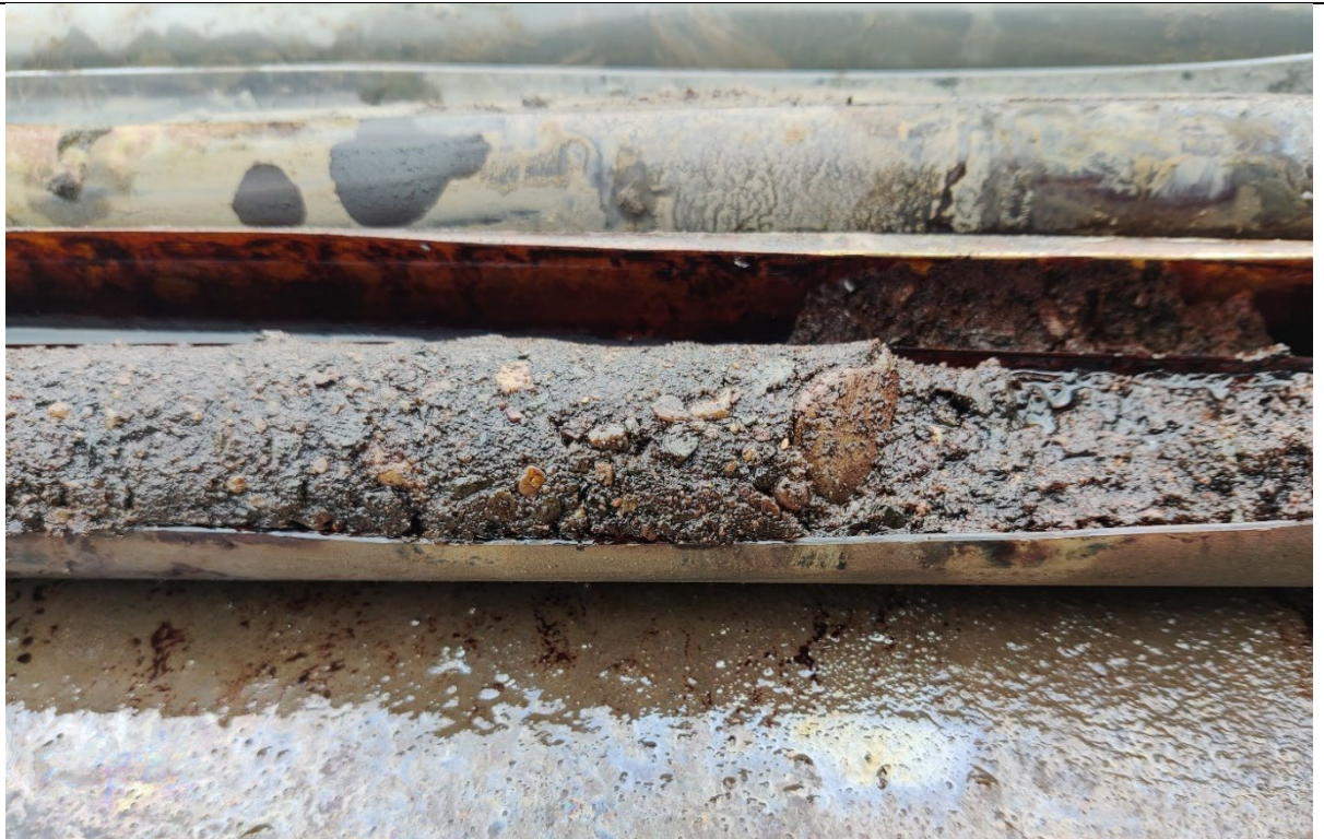
Photo 2- Representative photo of boring DB-21 which is impacted with MGP Coal Tar at the 35-40' interval
