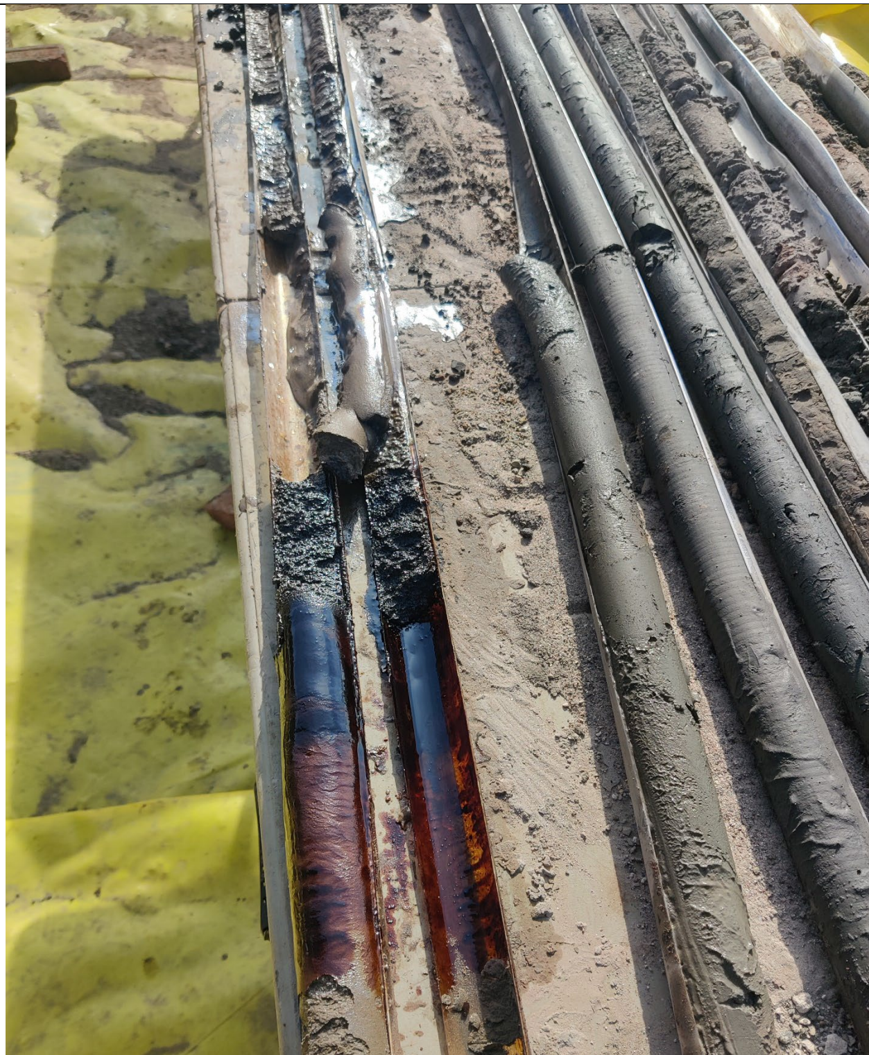
Photo 3- Photo of boring DB-25 impacted with MGP Coal Tar at the 60-65' interval.
