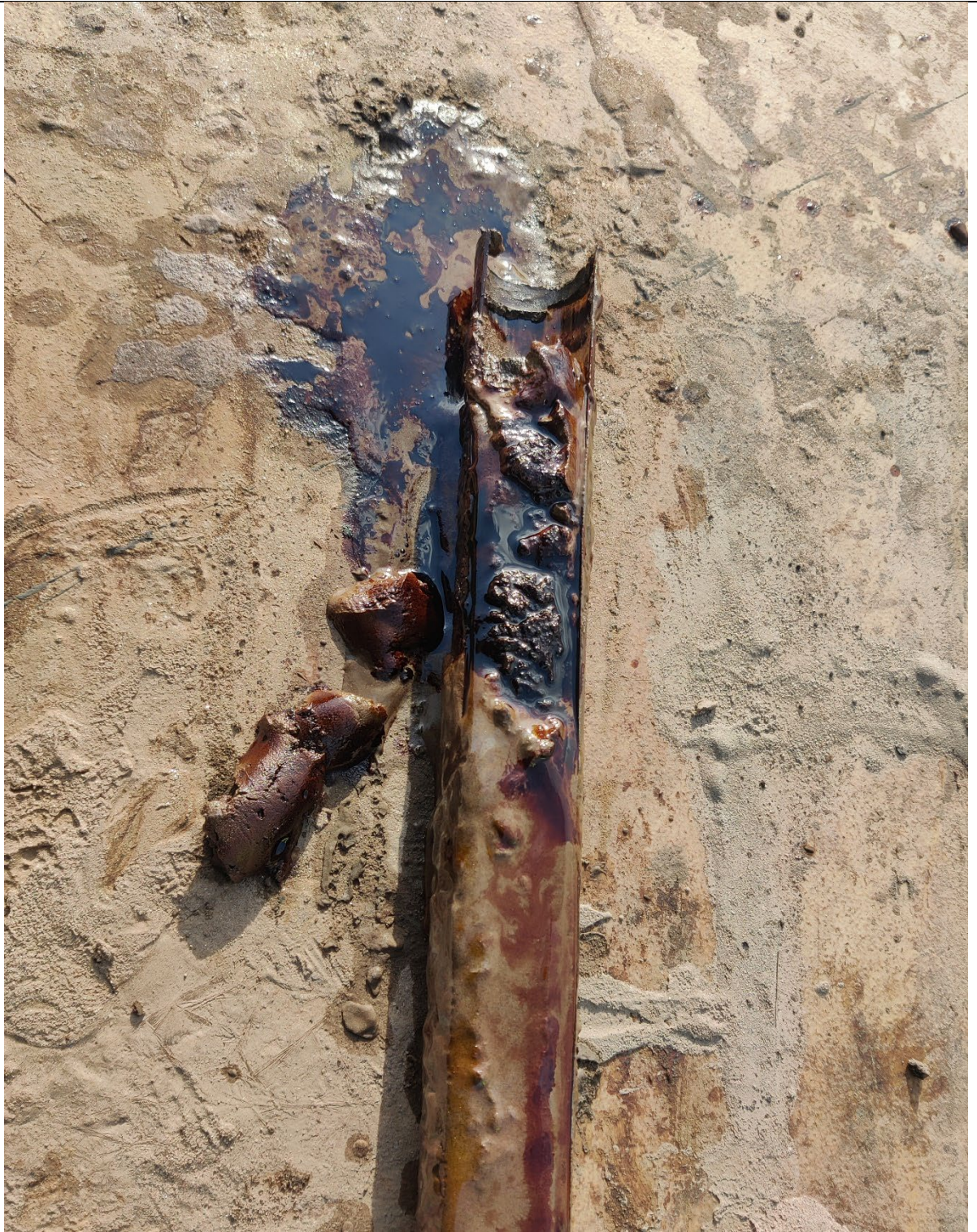
Photo 2- Representative view of material impacted with MGP Coal Tar at boring DB- 25, within the 60-65' interval.
