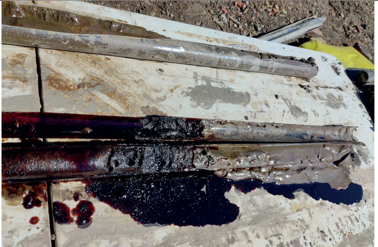
Photo 2- Representative view of boring DB-11, impacted with MGP coal tar at the 40-45' interval.
