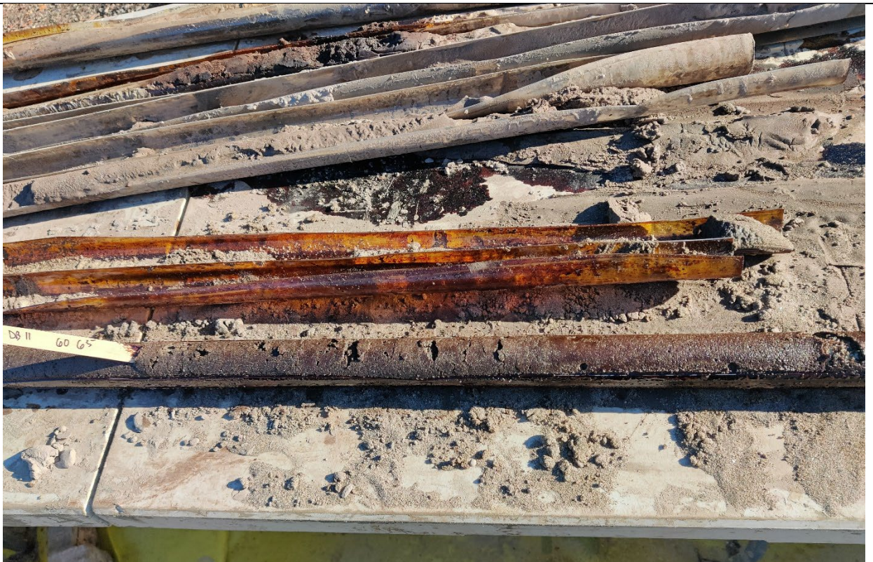
Photo 2- Representative view of boring DB-11 impacted with MGP Coal Tar at the 60-65' interval.
