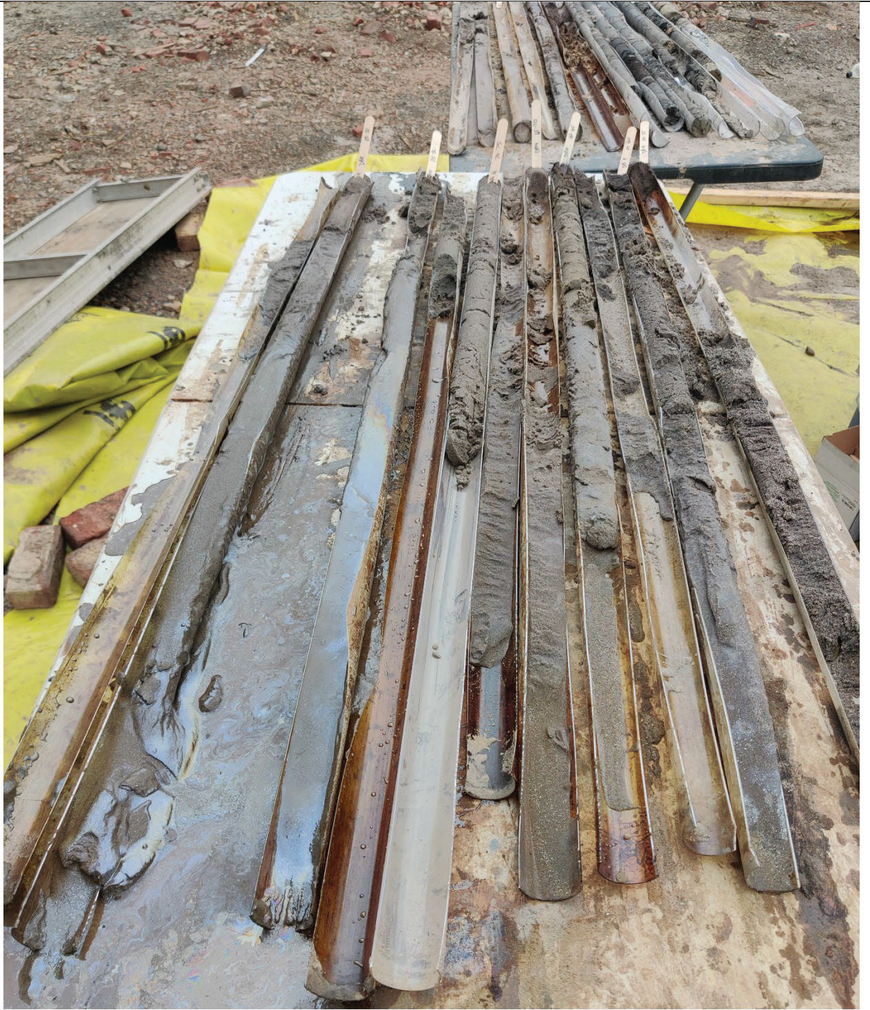
Photo 3- Representative view of boring DB-4, impacted with MGP Coal Tar at the 50-85' interval (right to left).
