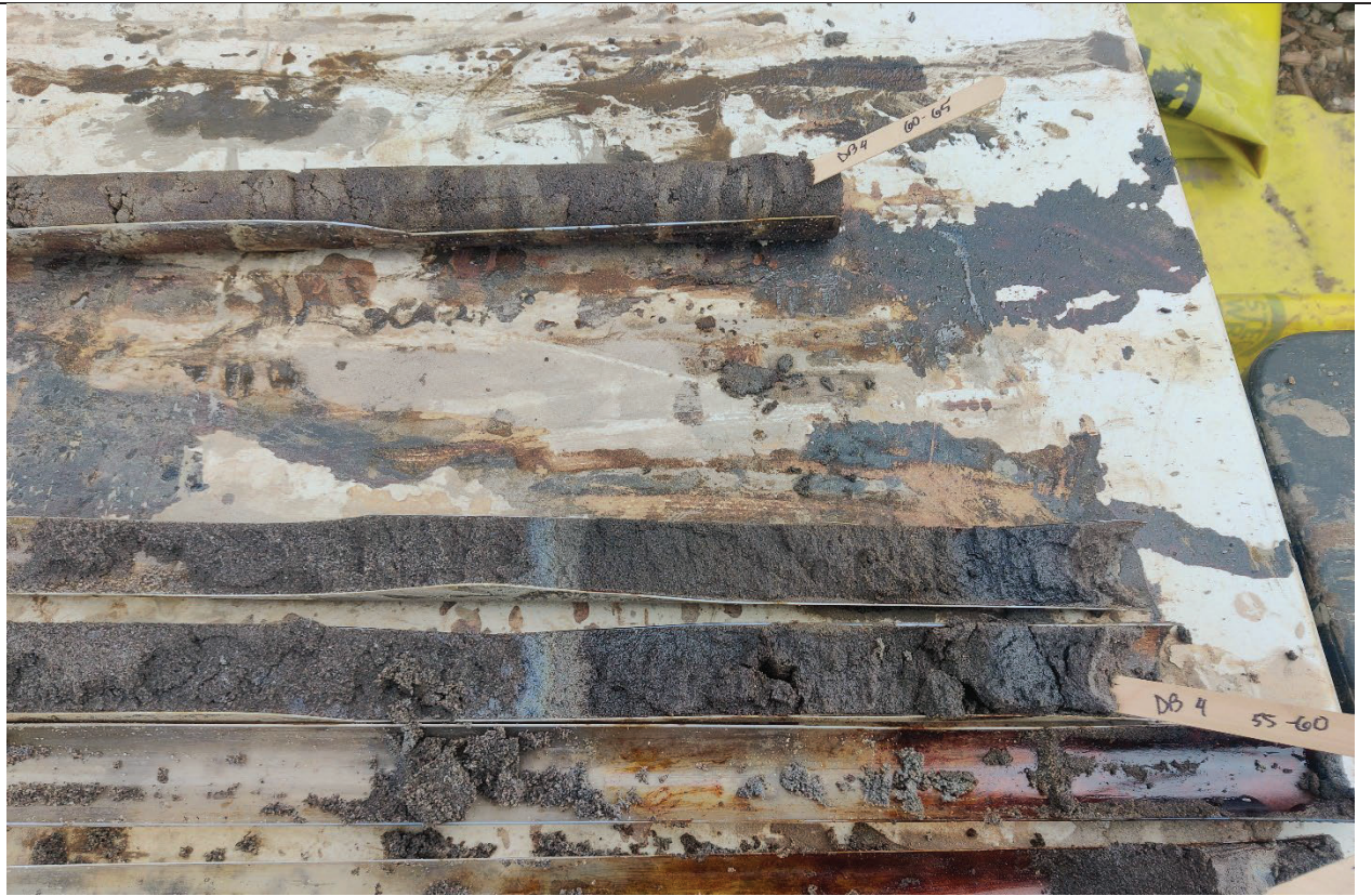
Photo 2- Representative view of boring DB-4, impacted with MGP Coal Tar at the 55-60' interval.
