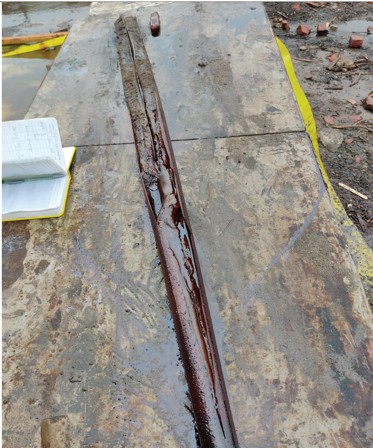
Photo 5- Representative view of boring DB-29, second interval of MGP coal tar observed from the 50-55' interval.
