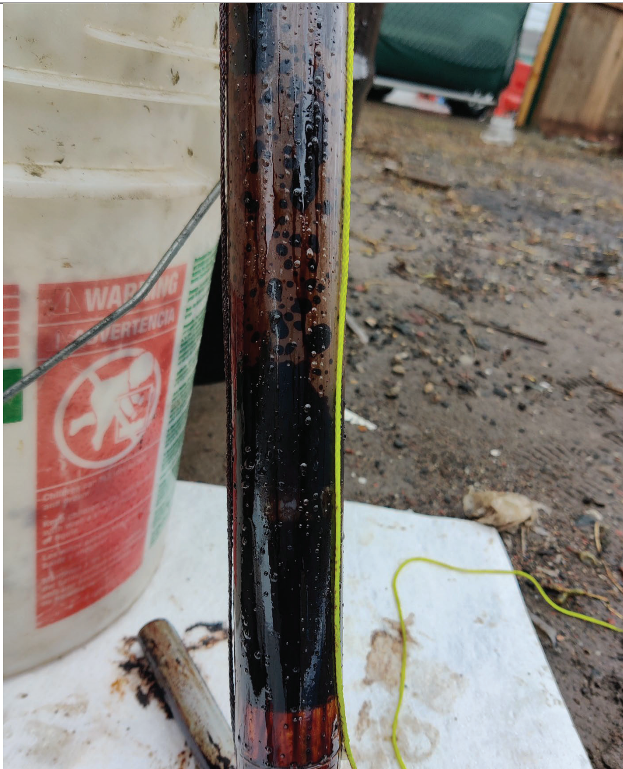
Photo 3- Additional Photo of MGP coal tar within bailer of intermediate cluster well GW-8.
