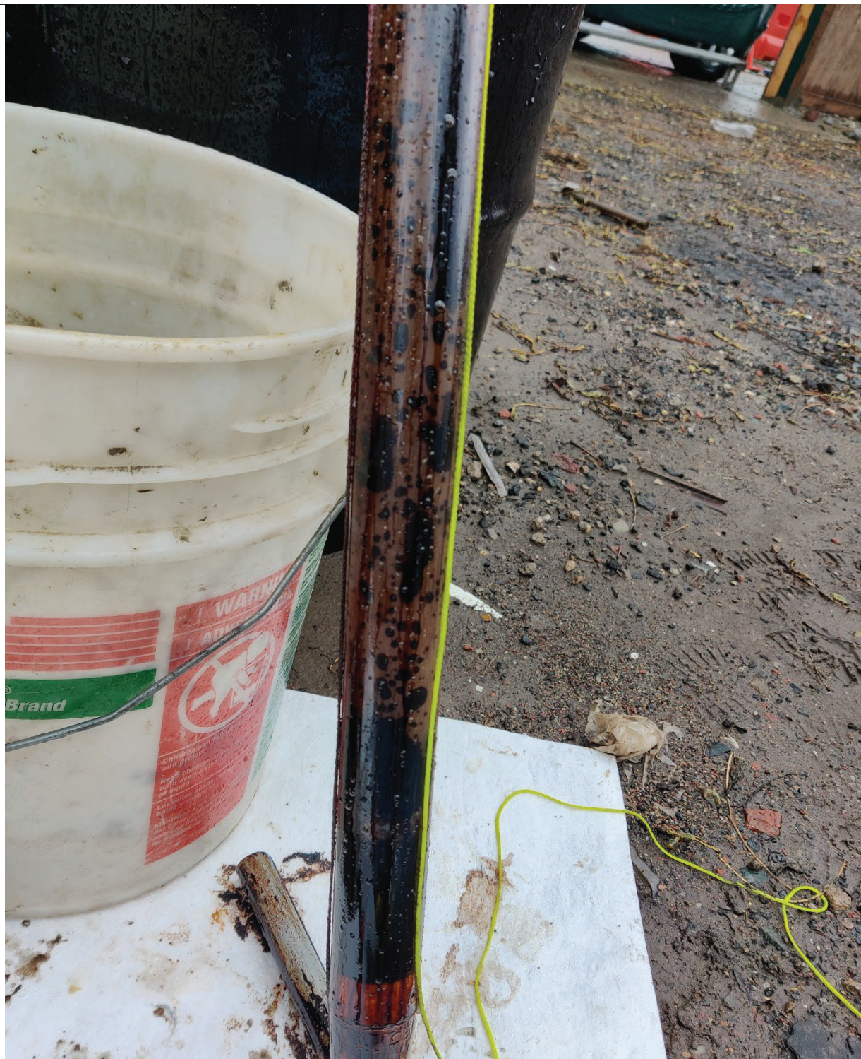
Photo 2- View of cluster well: GW 8, the intermediate cluster well with a sump from 45-50-feet bgs. At least 5-6 inches of MGP coal tar collected in the bottom of the bailer, as pictured.
