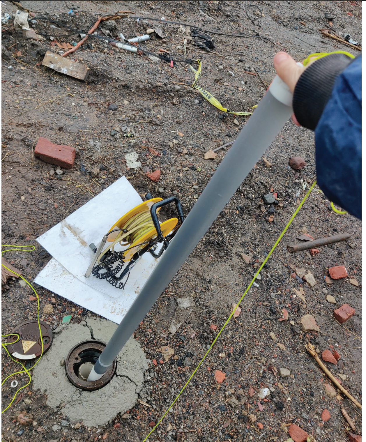
Photo 3- View of bailer pulled from cluster well: GW-8, the deep cluster well installed to 92-eet bgs. No MGP coal tar was observed in this cluster well.
