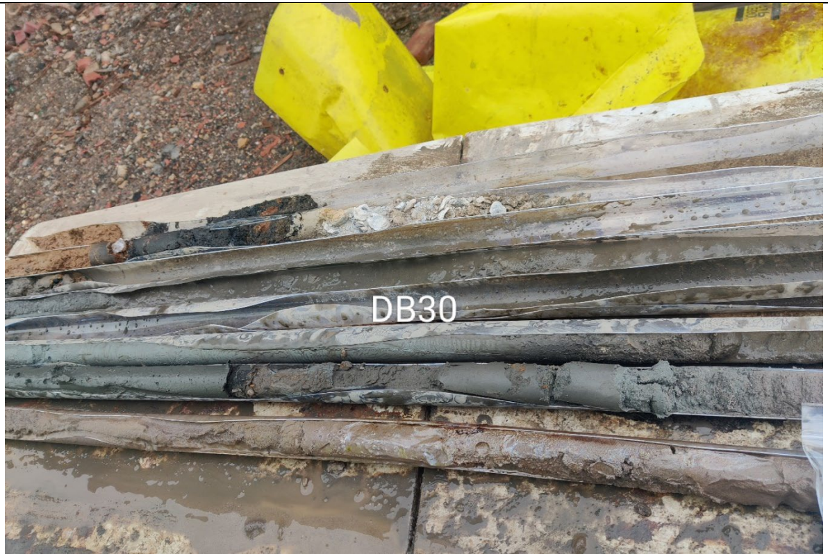
Photo 3- View of boring DB-30, a small interval of MGP Coal Tat was identified at the 32' interval.
