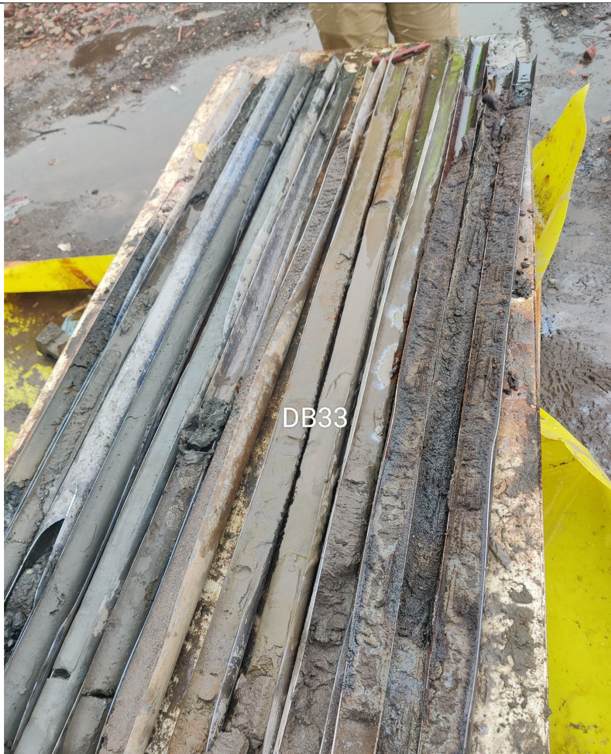
Photo 2- View of boring DB-33, intervals 0-60-foot bgs, left to right. MGP Coal Tar identified at 50 feet.
