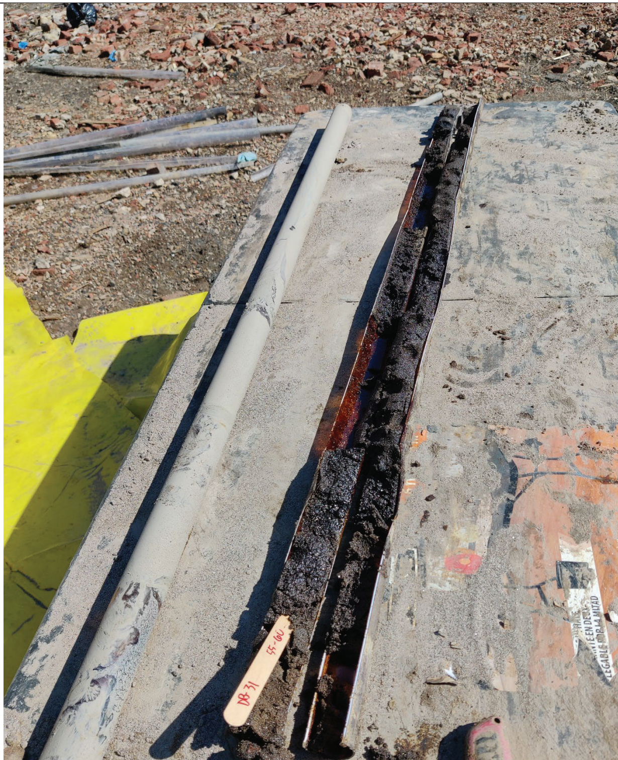
Photo 3- Representative view of boring DB-31 impacted with MGP Coal Tar at the 55-60' interval.
