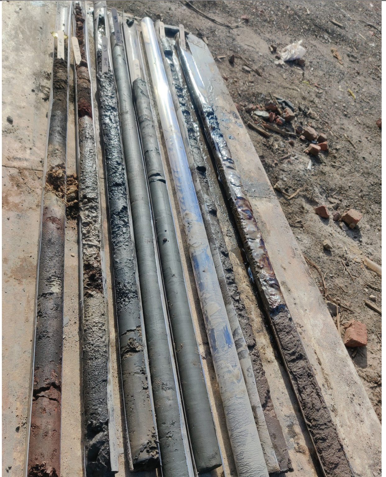
Photo 2- View of boring DB-3 from grade 40-foot bgs. MGP coal tar observed at the 35-40' interval.
