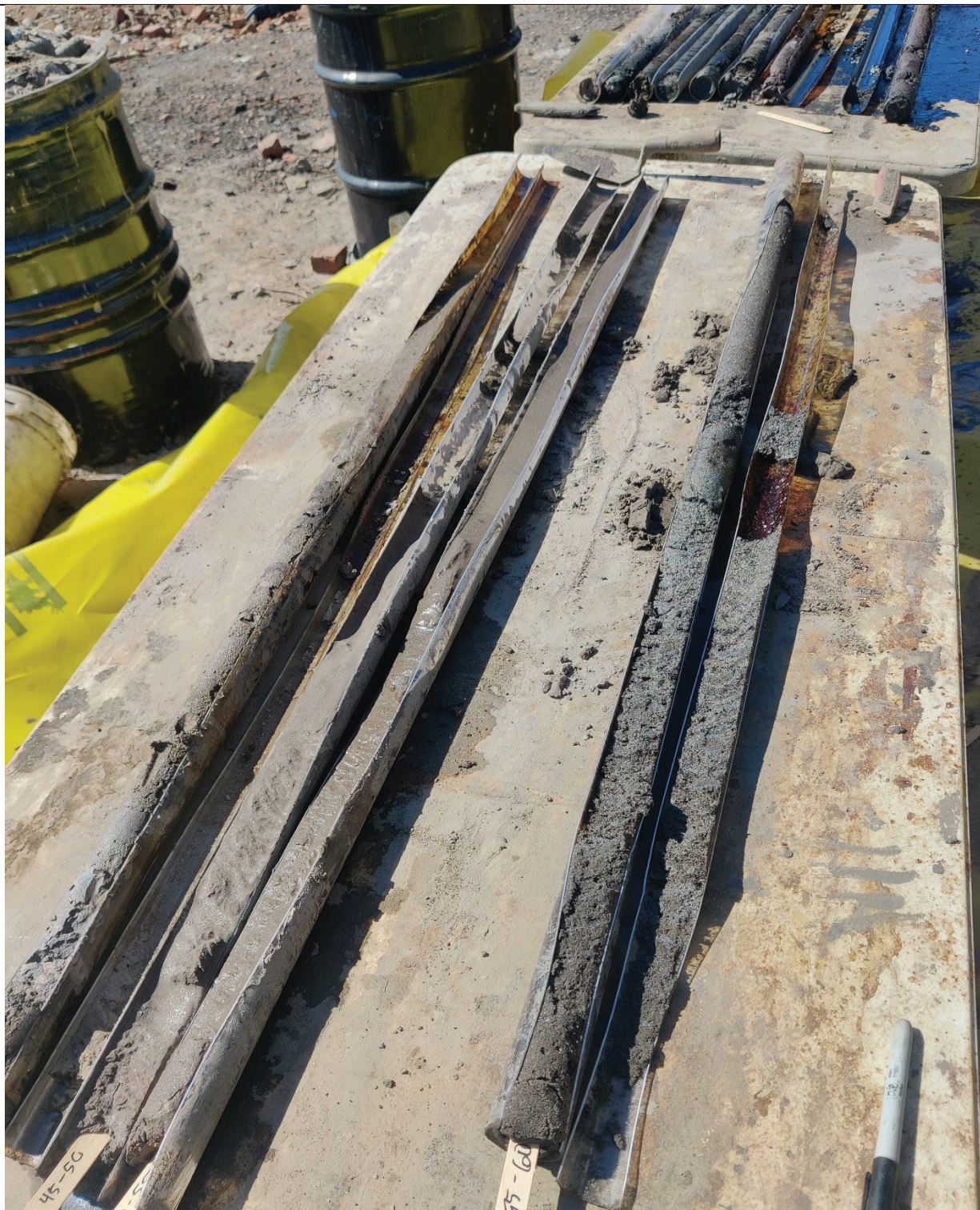
Photo 4- View of boring DB-9 at the 55-60' interval, impacted with MGP coal tar.
