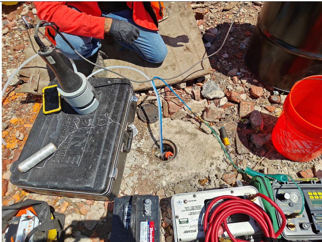
Photo 2- Representative picture of low flow groundwater sampling in progress.
