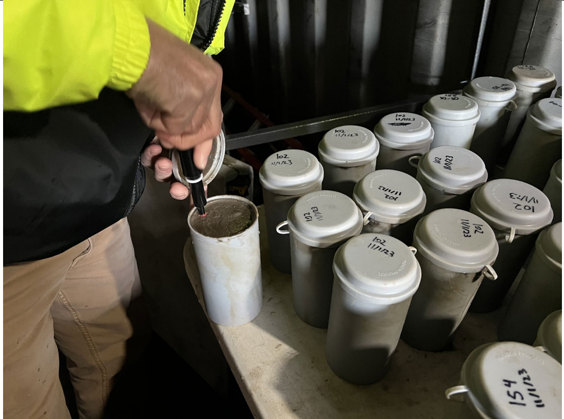
Photo 1- Representative photo of Cascade conducting a penetrometer test.
