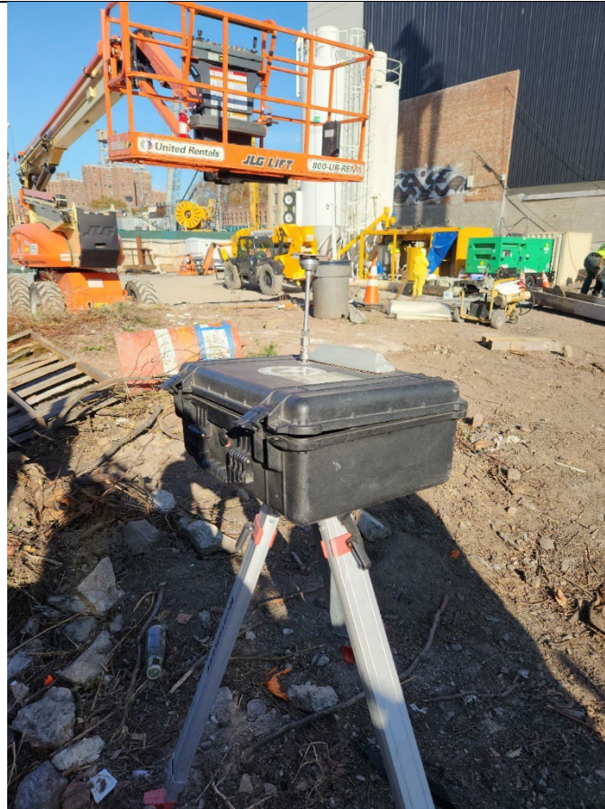
Photo 3- Representative view of CAMP unit set up.
