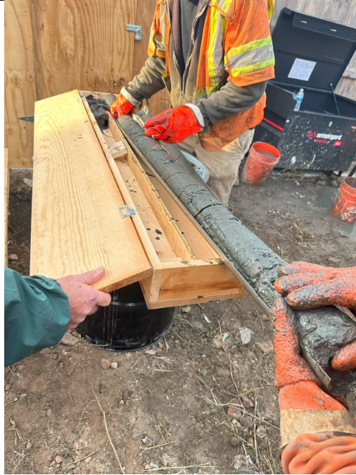
Photo 1- Representative photo of core sample from Pile 25 (Mix C) from the 5 to 10-foot interval.
