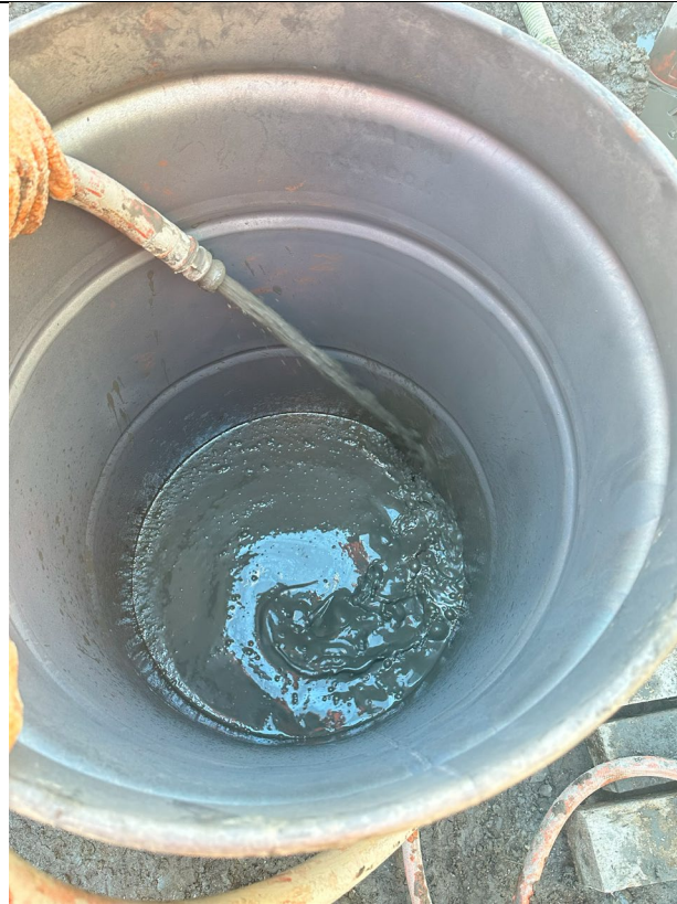
Photo 3 – Representative view of ADT pumping water into drums, after completion of core sampling.
