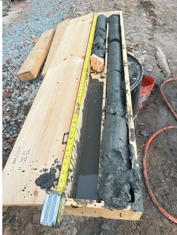
Photo 3 – Representative view of core samples at the 20-25-foot bgs and 2 to 30-foot bgs intervals of overlap core for Columns 304 and 337.
