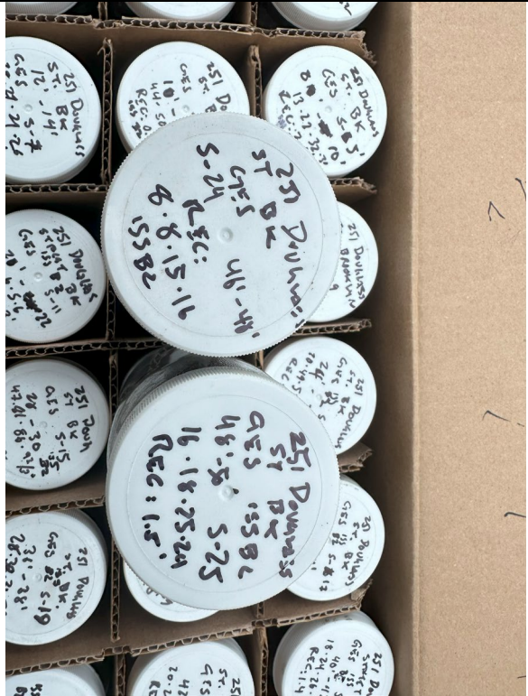
Photo 4 – Representative photo of split spoon soil samples from boring at Mix A.
