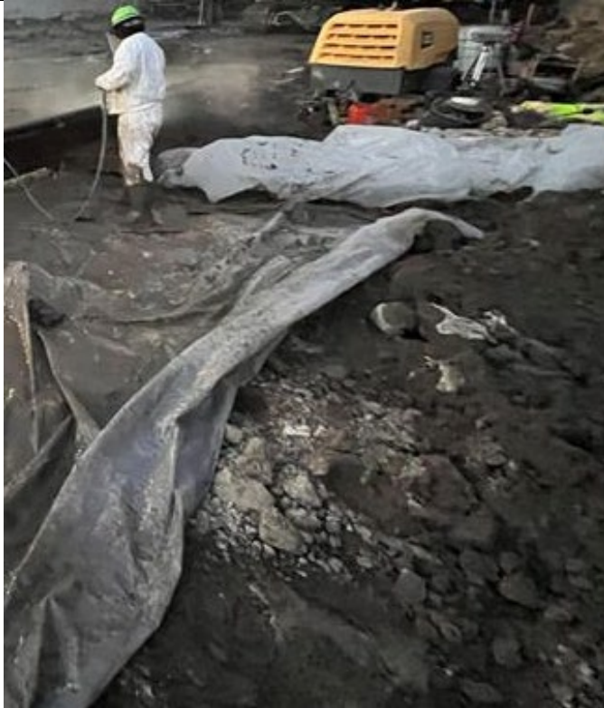
Photo 3- Representative photo of Cascade decontaminating the sampling rod.
