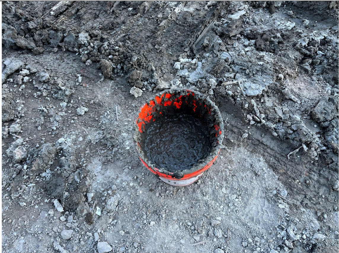
Photo 4- Representative photo of the wet mix sampled collected from Column 103.
