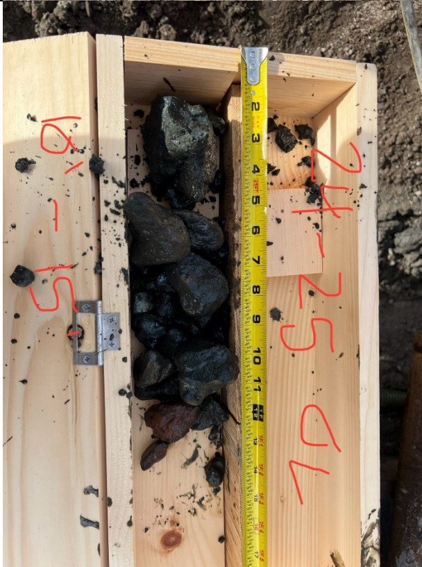
Photo 2- Representative photo of a OL core recovered, note poor recovery.
