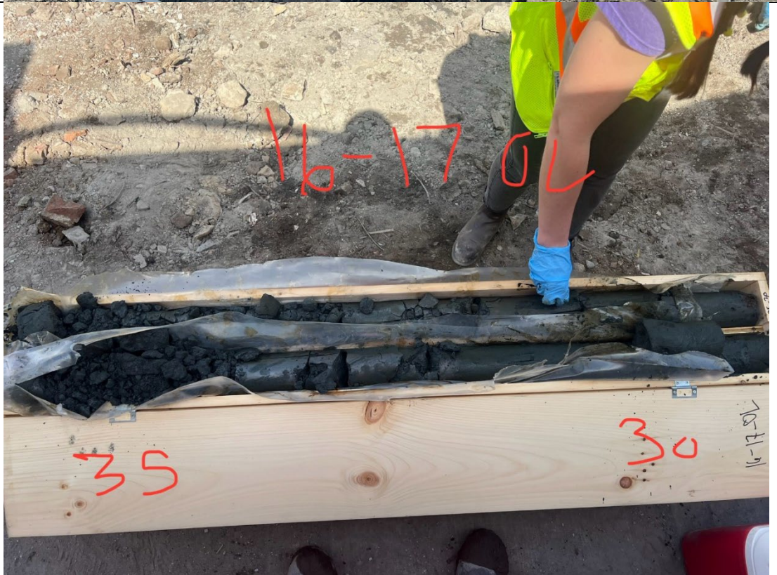
Photo 4- Representative photo of an ISS full scale column core.
