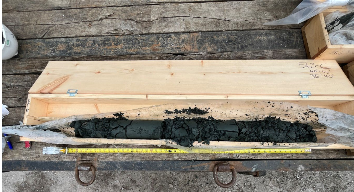
Photo 4- Representative photo of ISS column core.
