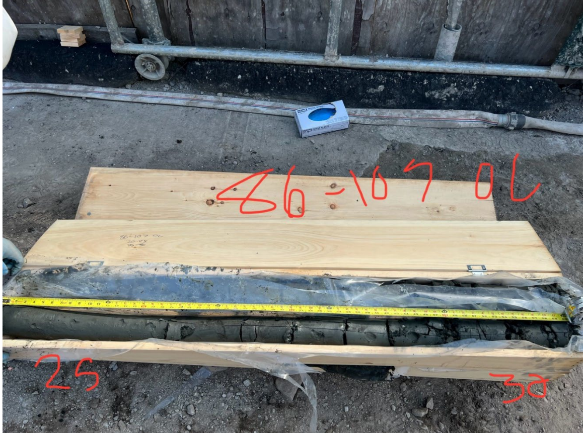
Photo 2- Representative photo of a QA/QC core from a full scale ISS column.
