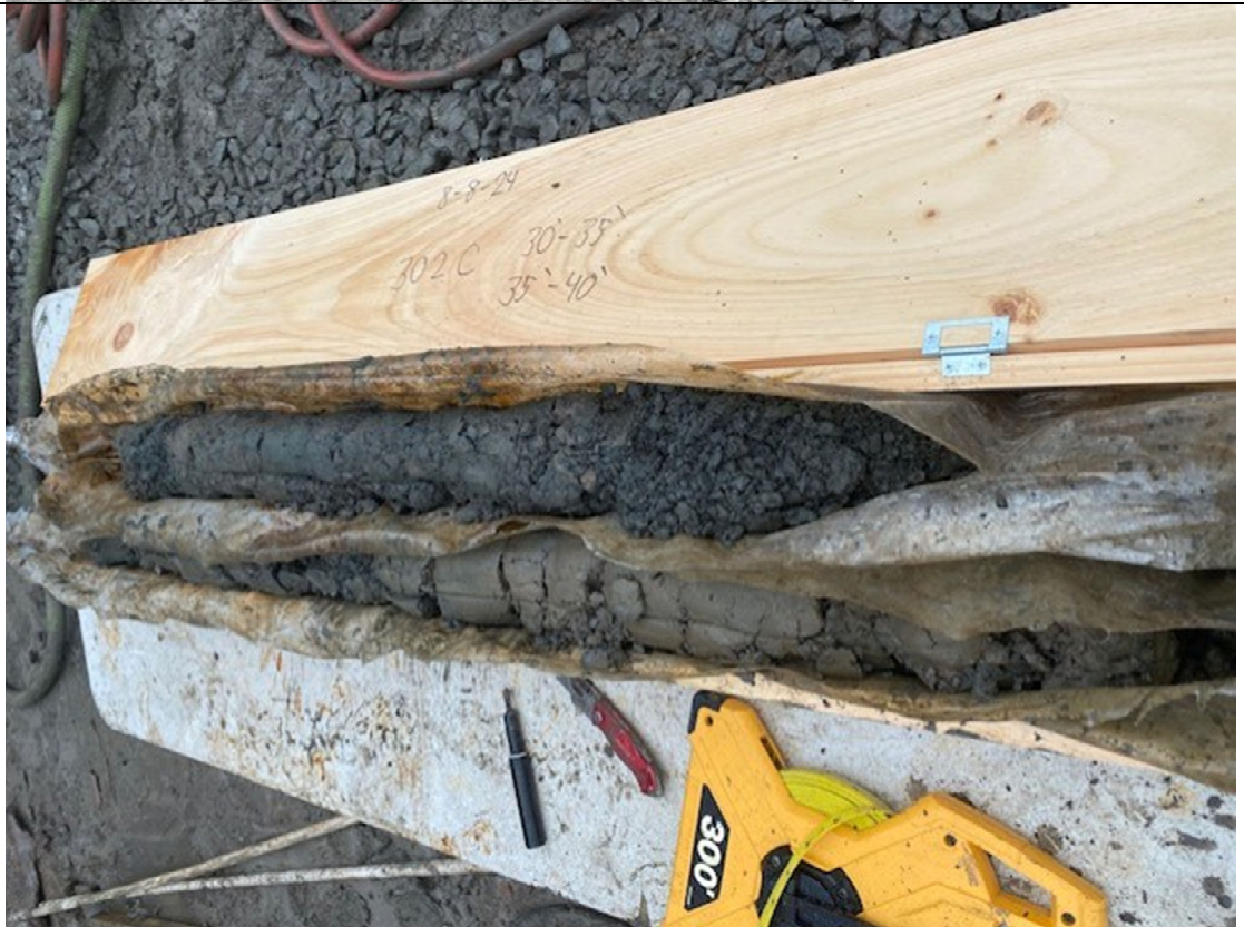
Photo 6- Representative photo of a QA/QC core from the ISS pilot test.
