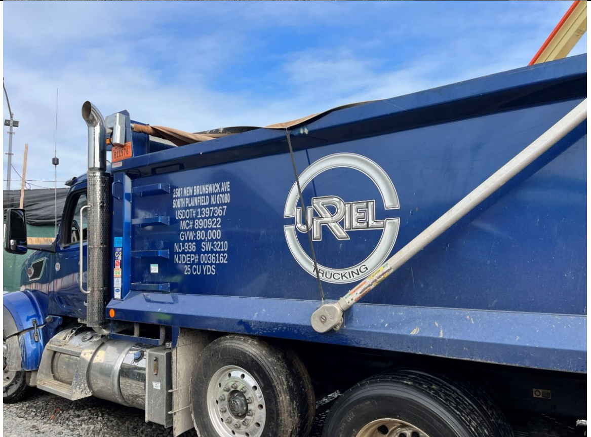
Photo 4- Representative photo of swell truck cover strapped down securely.
