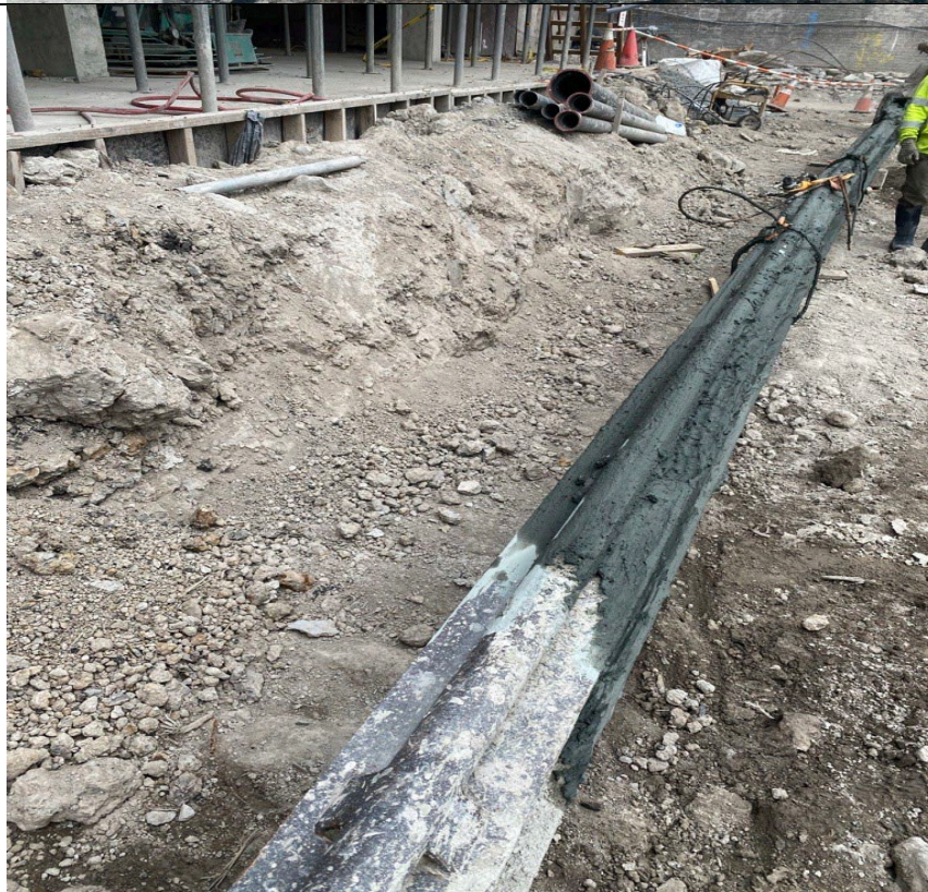
Photo 2- Representative photo of bar used to collect wet-mix sample from 30' depth on Column 304.
