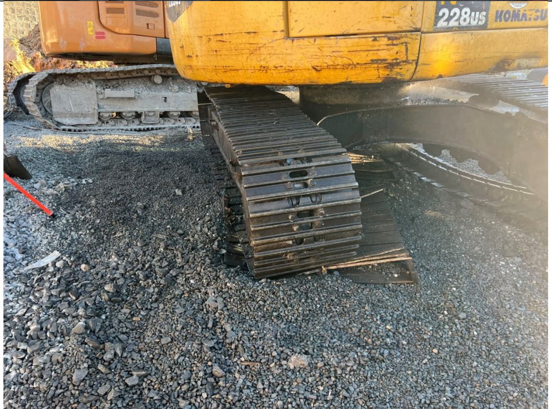
Photo 4- Representative photo of clean excavator tracks before excavator bringing it on the street.
