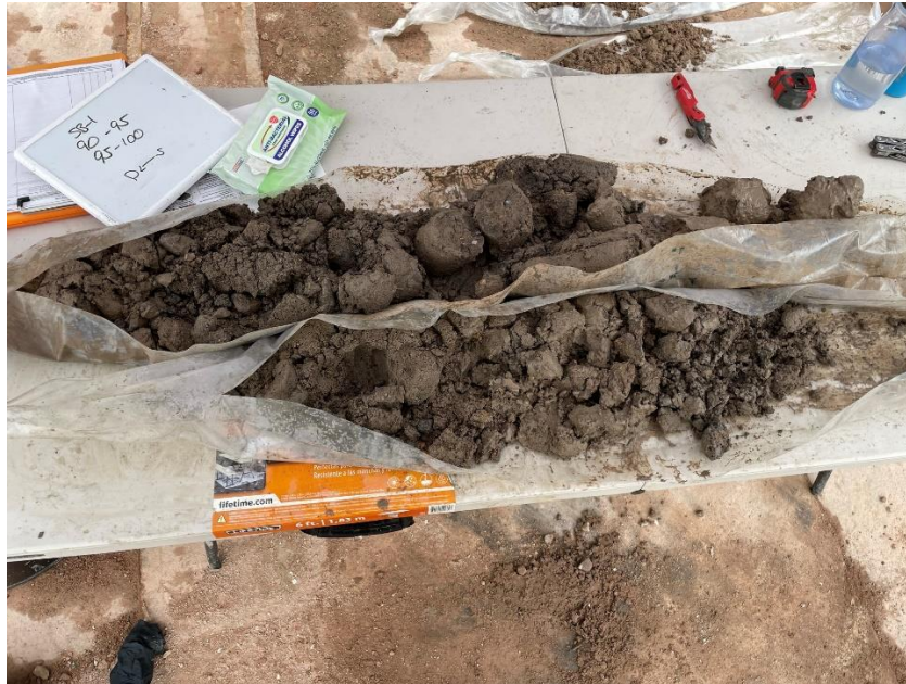
Photo 1: Soil from SB-1 from 90-100 ft bgs, facing east.
