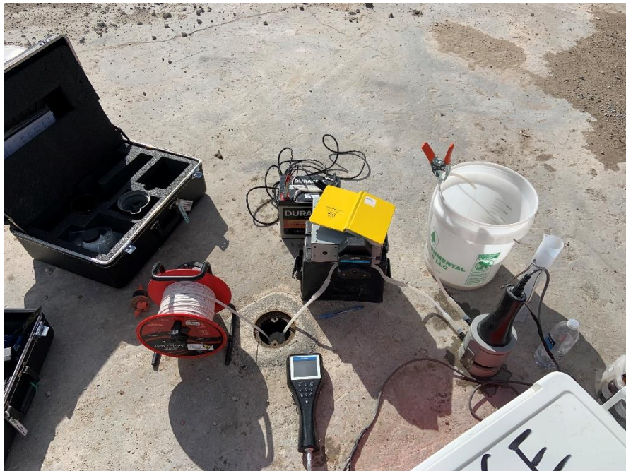
Photo 2: View of low-flow sampling, facing north.
