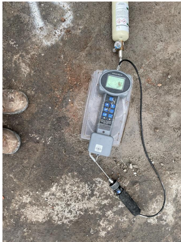
Photo 2: Helium Shroud fit test on SV-7, facing south.
