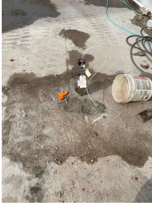
Photo 1: Soil vapor collection at SV-3, facing south.
