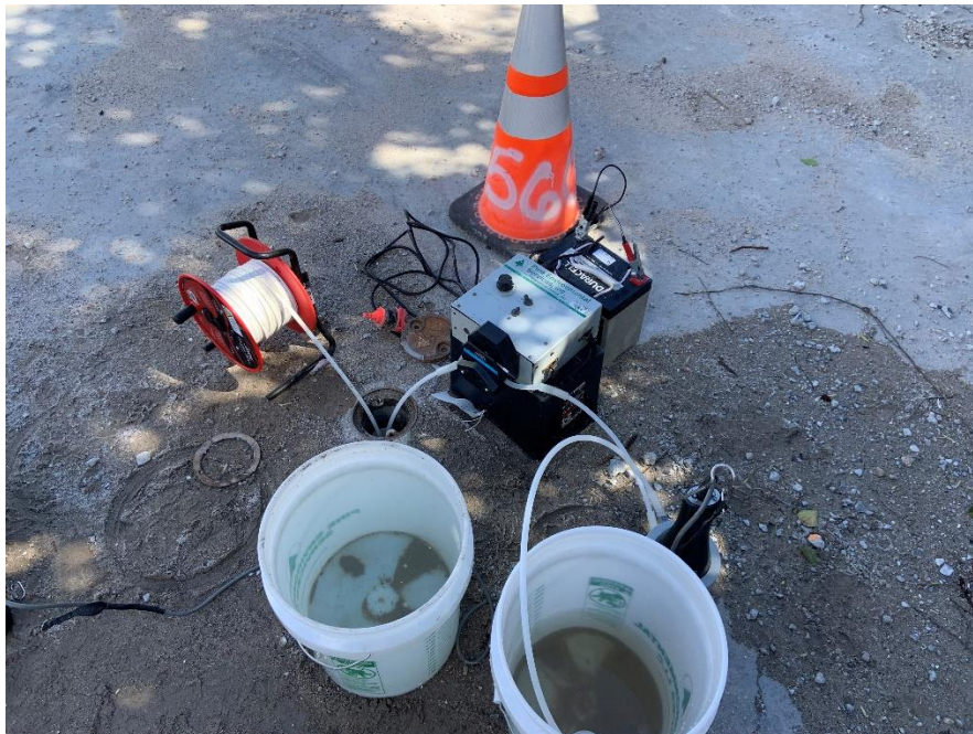
Photo 2: View of low-flow sampling, facing south.
