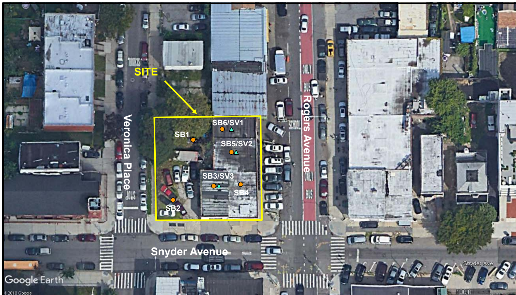
FIGURE 2 – SOIL BORING AND SAMPLE LOCATION MAP
