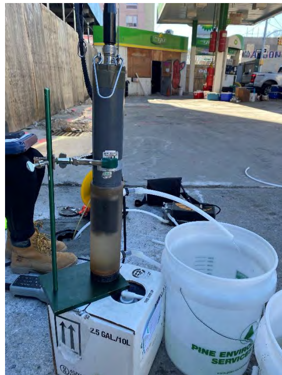
Photo 2: View of MW-05 groundwater sampling activities.
