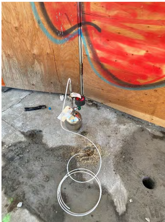
Photo 2: View of VP-02 soil vapor sampling activities.
