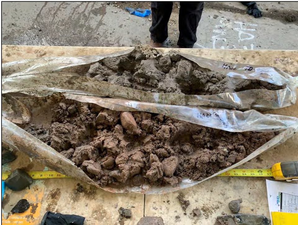
Photo 2: View of 90 to 100 ft bgs interval of deep soil boring HA-22.
