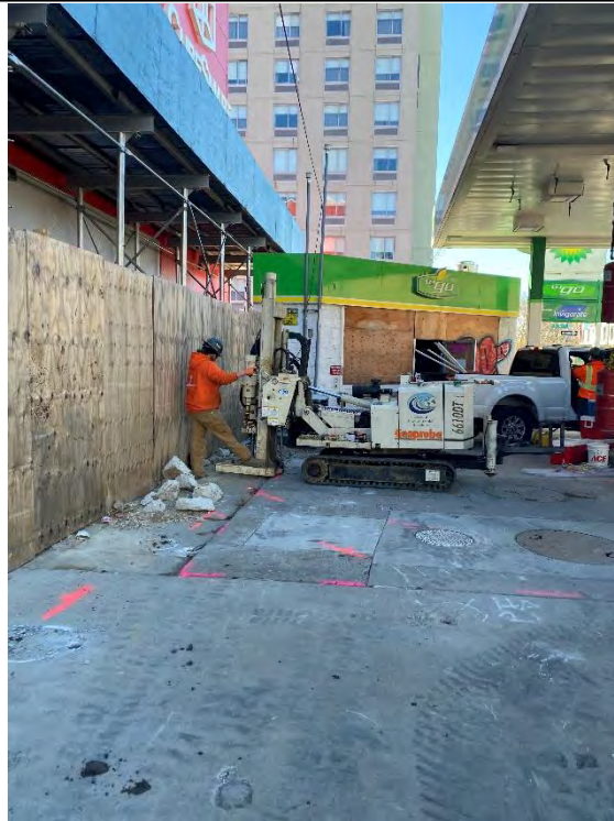
Photo 1: View of HA-26 soil boring drilling activities.
