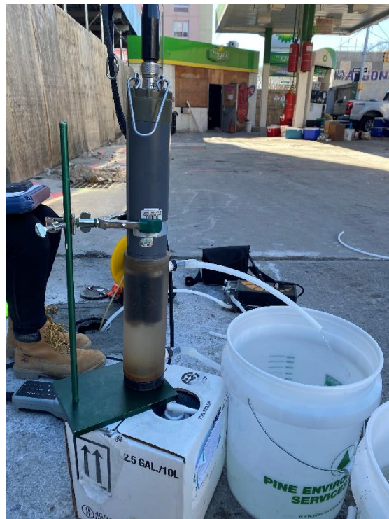
Photo 2: View of MW-05 groundwater sampling activities.
