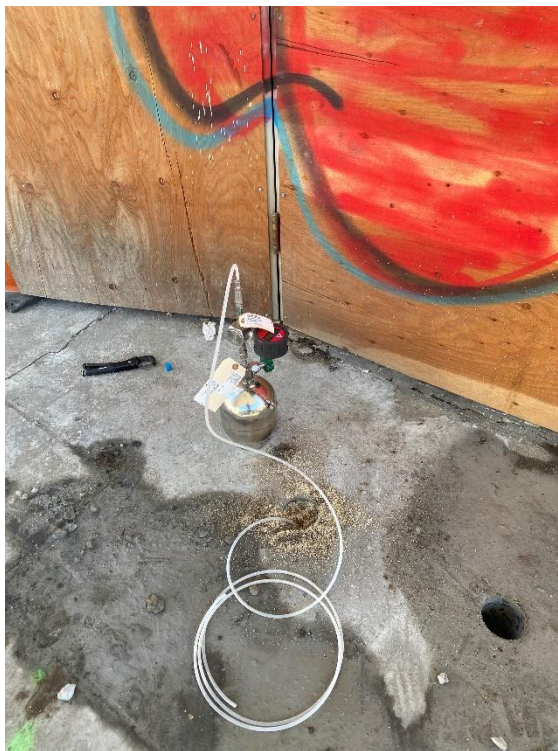
Photo 2: View of VP-02 soil vapor sampling activities.
