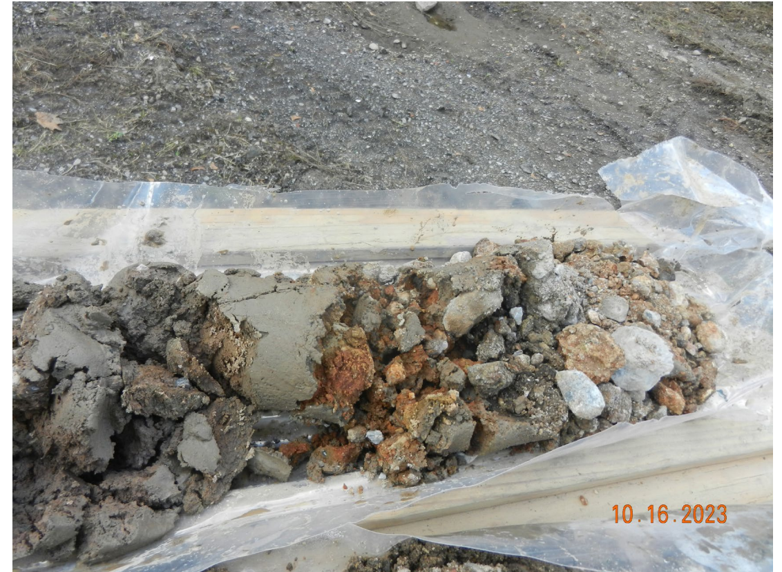
Soil sample at SB-7 at 31.50'-33.00' depth. Dark brown sand with gravel.
