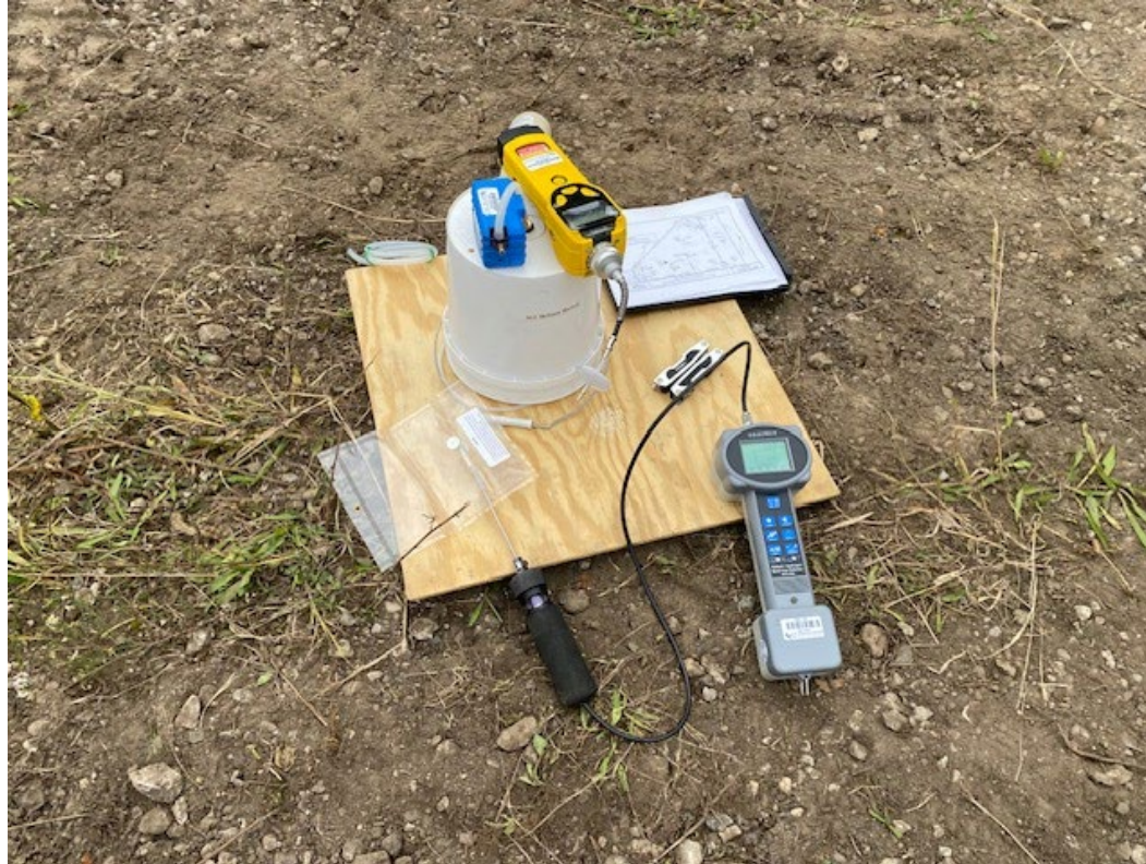
Checking the soil vapor sampling point for VOCs with a PID (yellow instrument) and to ensure a good seal from the ambient air with the bucket, air sampling pump and the helium detector
