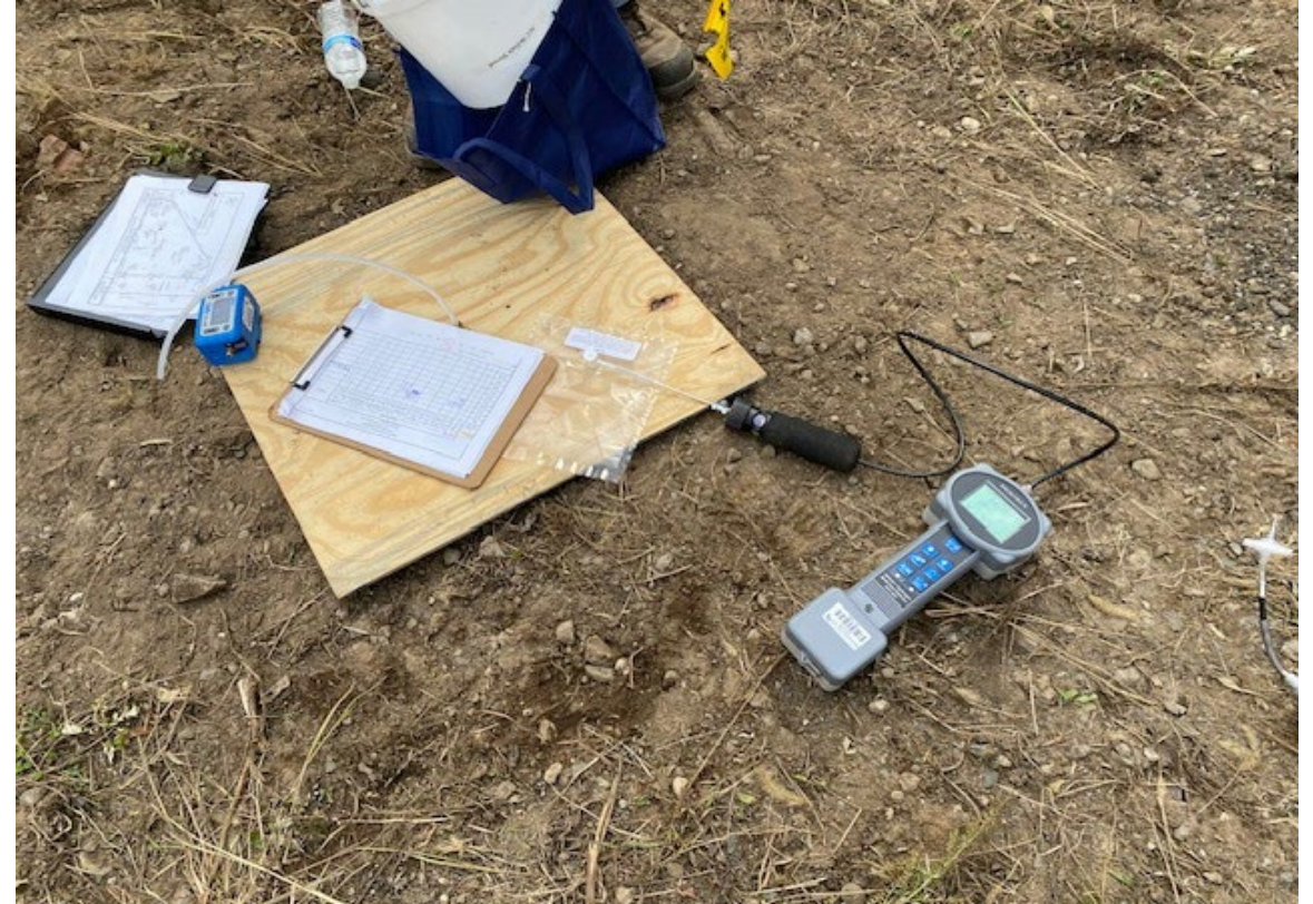
¼" diameter tubing from the soil vapor implant extended up through a piece of plywood to provide a solid and even surface to check the vapor implant seals.
