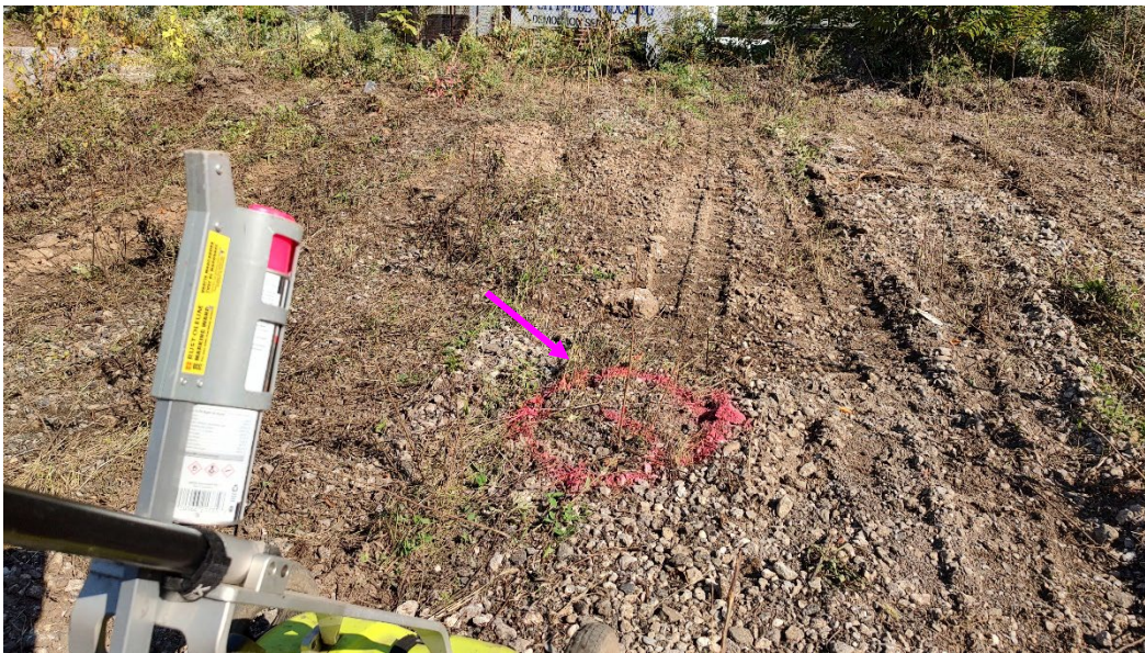
Photo 3 – View of one of the many metallic anomalies detected with the TW-6 Magnetometer which detects the presence of shallow metal objects. Upon further investigation with the GPR unit shown above, the anomalies were determined to be unremarkable.
