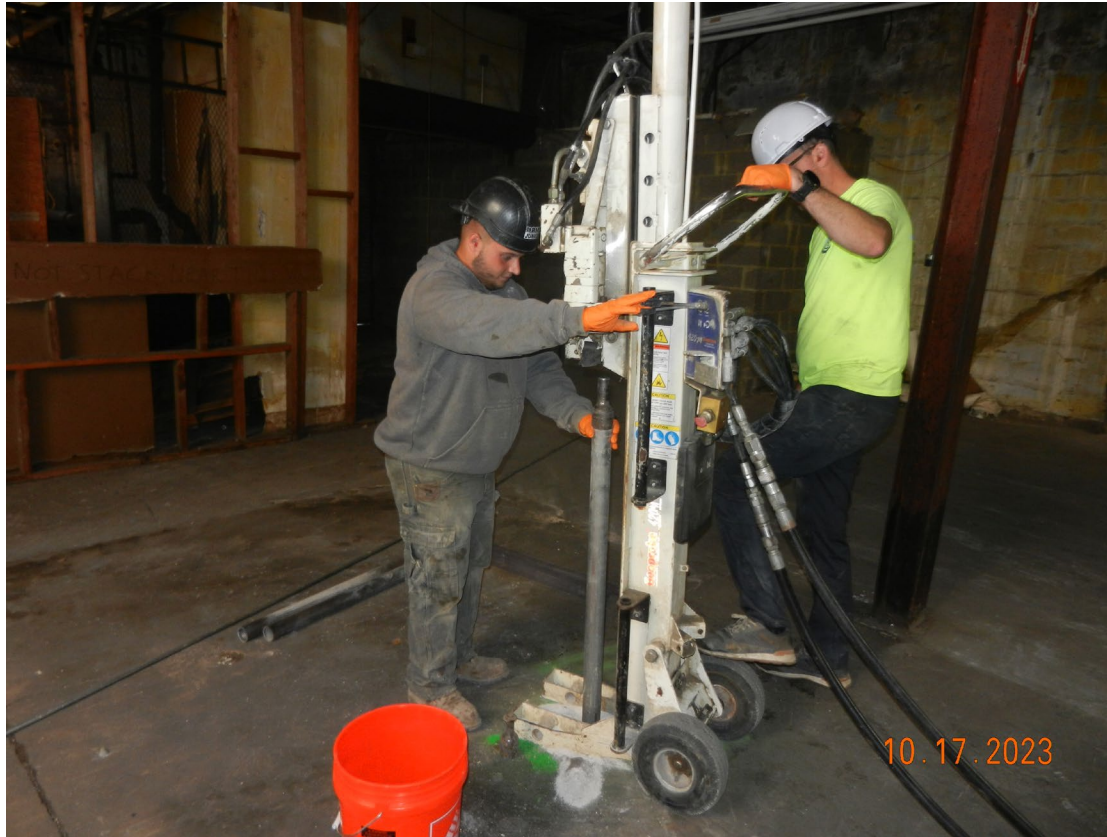
Attaching the 3 foot macro-core soil sampler onto the portable drilling equipment.
