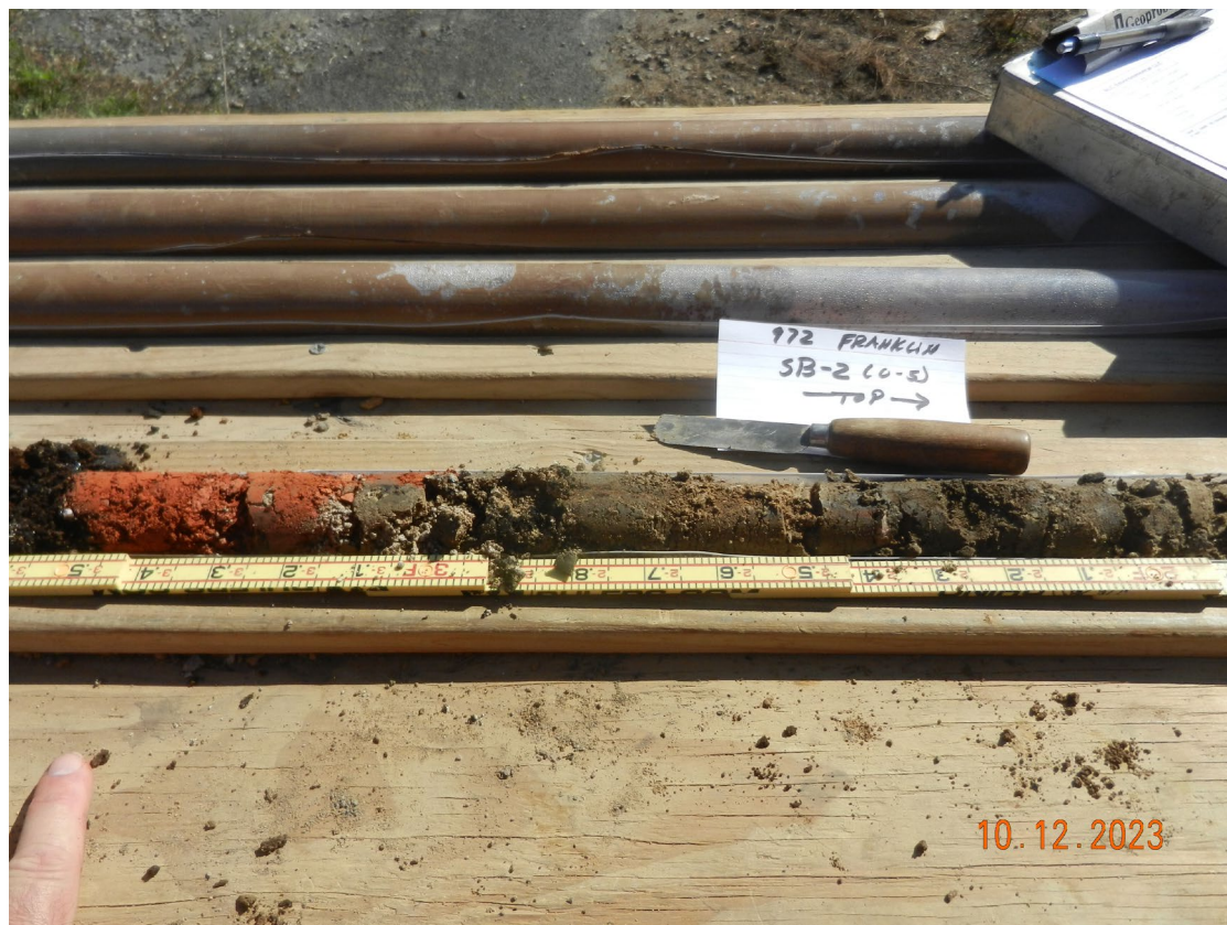
Soil Sample collected at SB-2 at 0'-5' depth. Moderate brown clayey sand with fill material (bricks & concrete).
