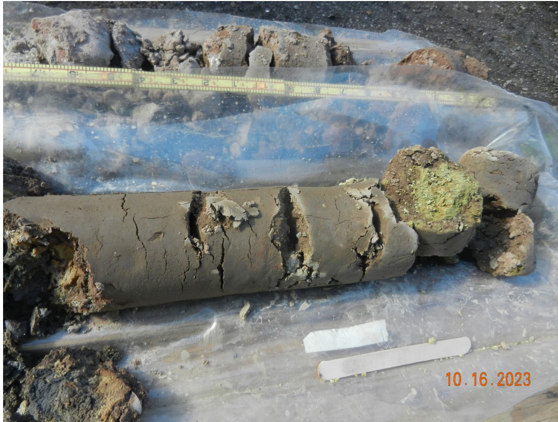
Soil sample at SB-7 at 30'-31.50' depth. Variegated light brown, dark yellowish brown and gray sandy clay with olive brown clayey fine sand.
