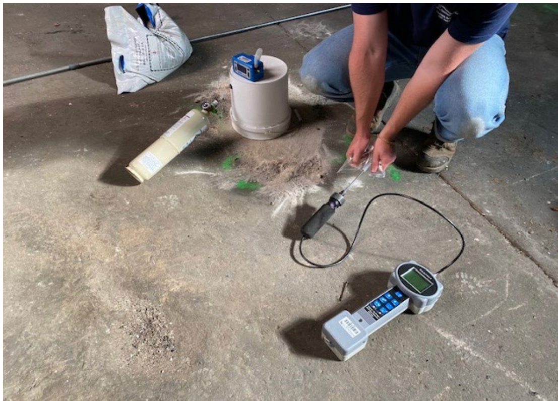
Checking the collected air sample in the tedlar bag for the presence of helium with the helium detector.
