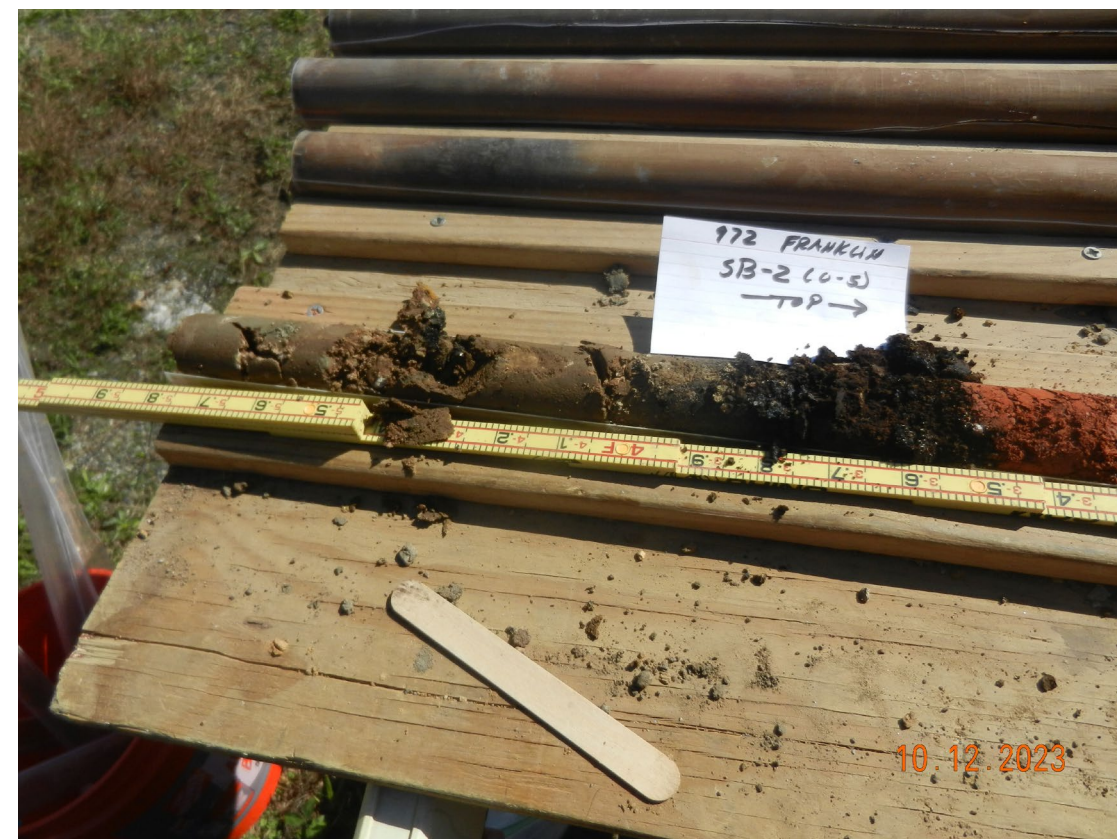
Bottom portion of the soil sample collected at SB-2 at 0'-5' depth. Medium gray micaceous sand.
