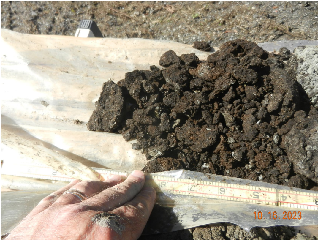
Soil sample at SB-7 at a depth of 30'-35'. Brownish gray clayey sand with brown peat.
