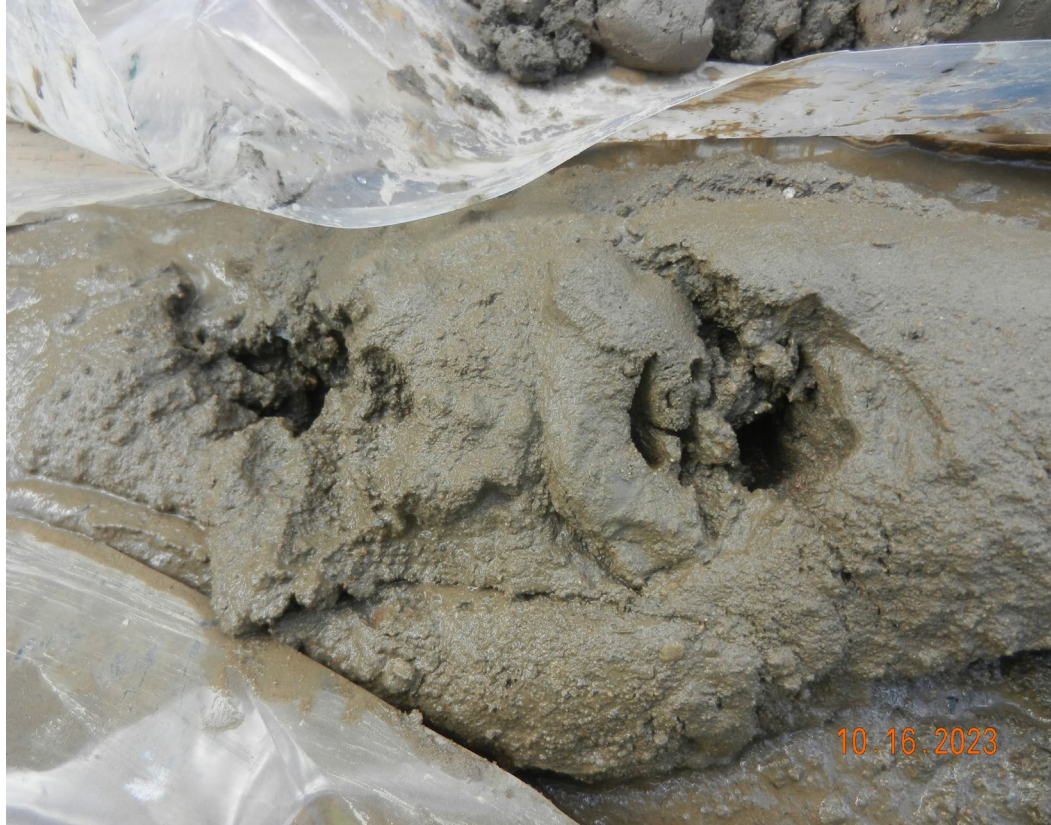
Soil sample at SB-7 at 45'-50' depth. Dark yellowish brown clayey sand with fine gravel, wet.
