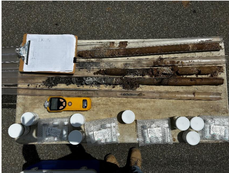
Photo 1: View of soil from SB-15 from 0-15 feet below grade surface, facing east.
